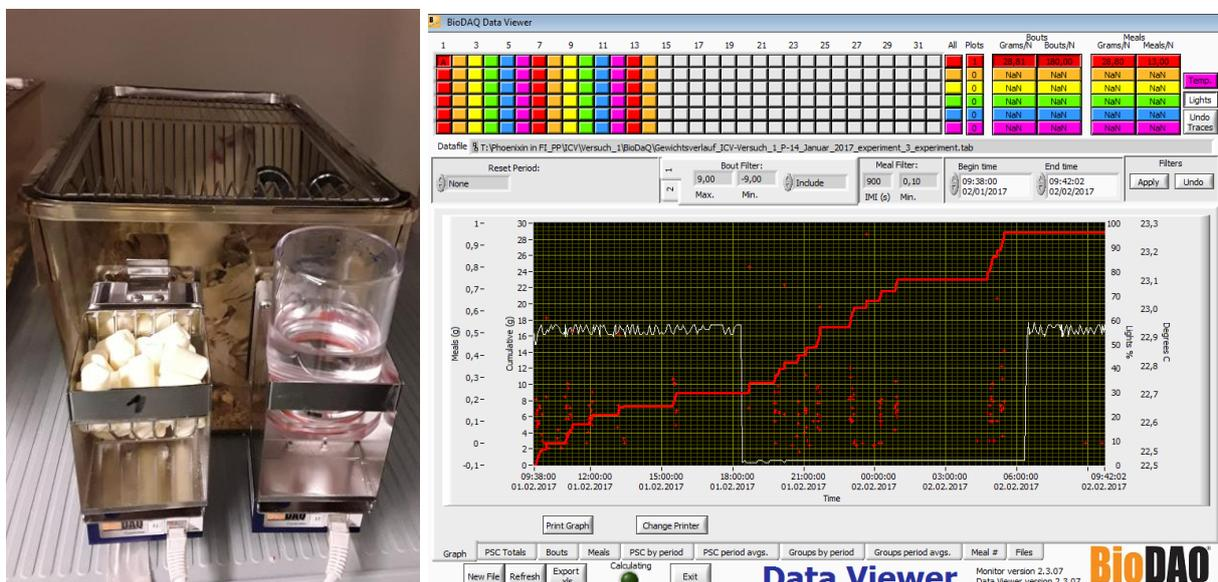
Figure 2: Automated food intake monitoring system.
