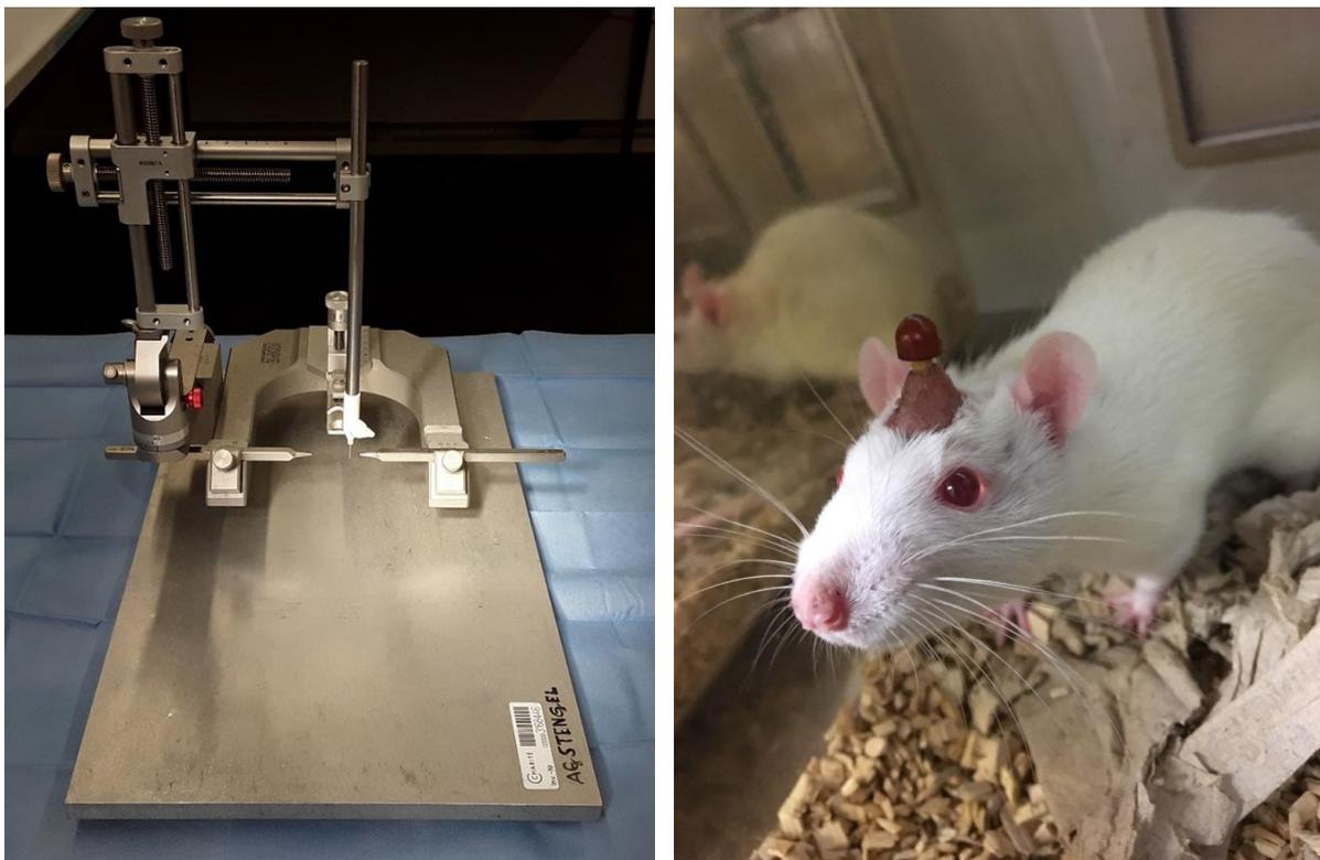
Figure 1: Stereotactic apparatus and intracerebroventricularly cannulated rat.
