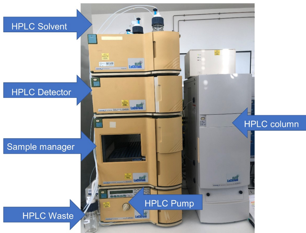
Figure 4. Basic components of an HPLC system
