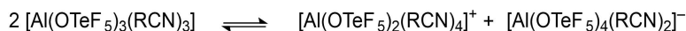
Scheme 3. Equilibrium between the neutral nitrile adduct of \text{Al}(\text{OTeF}_5)_3 and its autoionized ion-pair. (R = Me, Ph).
