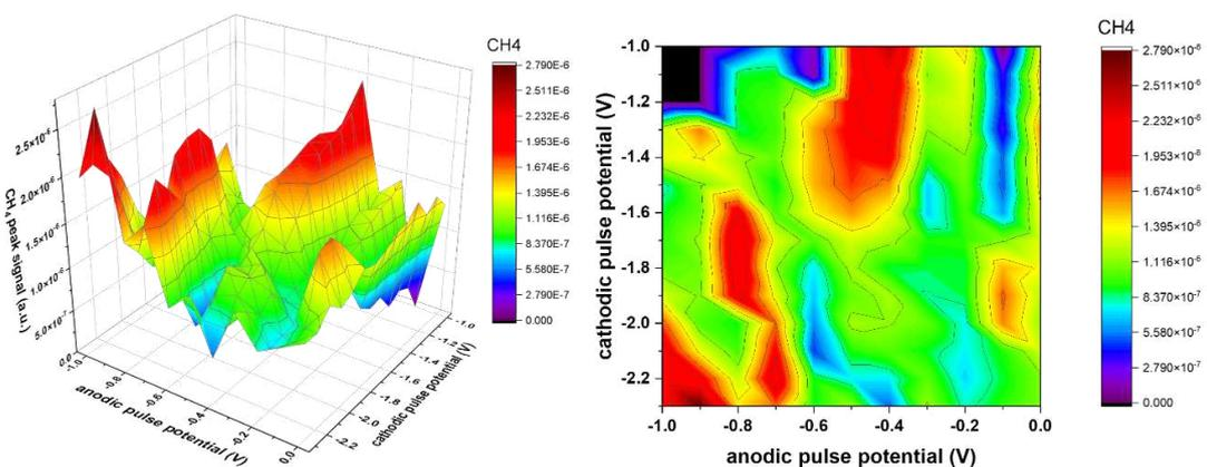
Figure 33: 3D and 2D plot showing the effect of pulse potential variation on CH<sub>4</sub>.
