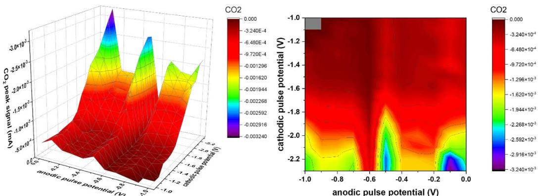
Figure 35: 3D and 2D plot showing the effect of pulse potential variation on  $\text{CO}_2$  signal.
