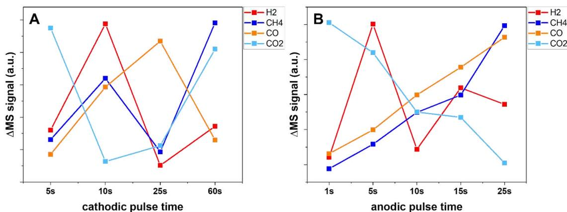
Figure 30: Averaged mass signal magnitudes over cathodic (A) and anodic (B) pulse time screening.
