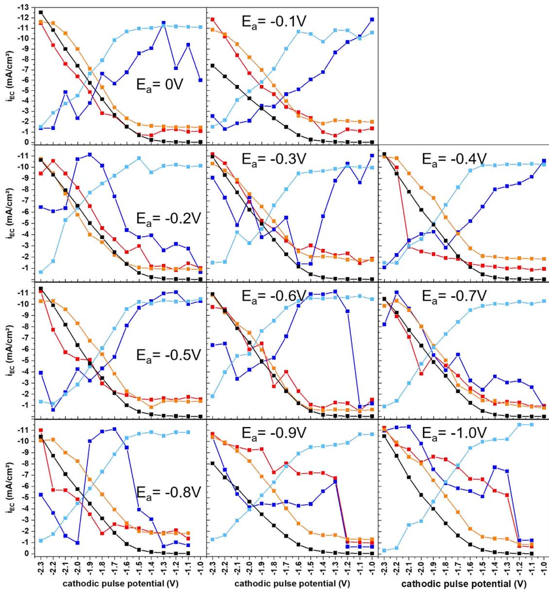
Figure 31: MS and current signal averages obtained at pulse potential screening with different fixed anodic pulse potentials. The y-axis shows a scalebar for the current density, while the mass signals are scaled in arbitrary units.
