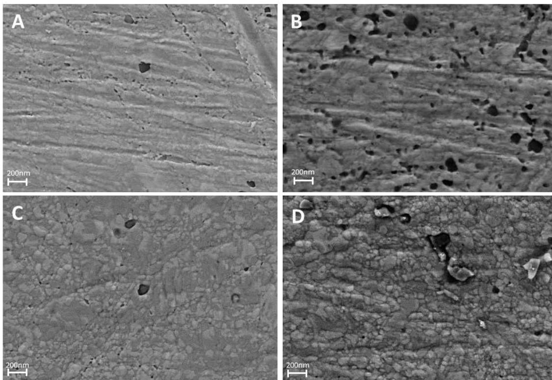
Figure 6: SEM images of silver foil samples before and after catalysis. A before, B after 7 h of potentiostatic catalysis at  $-2.1$  V, C after 3 h of pulsed electrolysis, D after 17 h of pulsed electrolysis at  $E_c = -2.15$  V,  $E_a = -0.5$  V,  $t_c = t_a = 5$  s.
