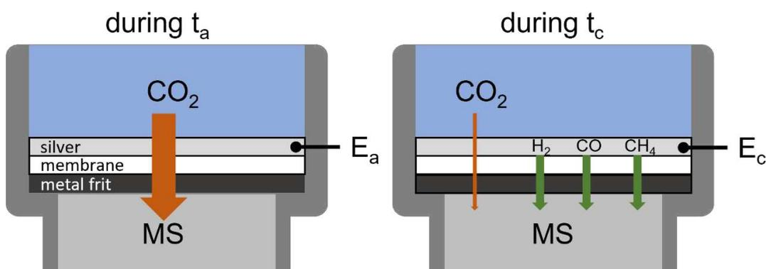
Scheme 4: DEMS cell scetch, visualizing gas flow during  $t_a$  and  $t_c$ .
