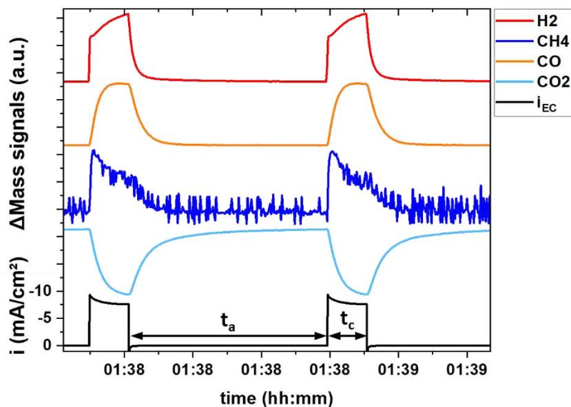
Figure 29: DEMS signals of major gaseous products formed under pulsed electrolysis at  $-2.1\text{ V}/-0.5\text{ V}$ ,  $5\text{ s}/25\text{ s}$ .
