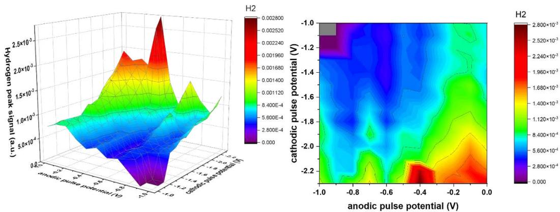
Figure 32: 3D and 2D plot of pulse potential screening data for H<sub>2</sub>.
