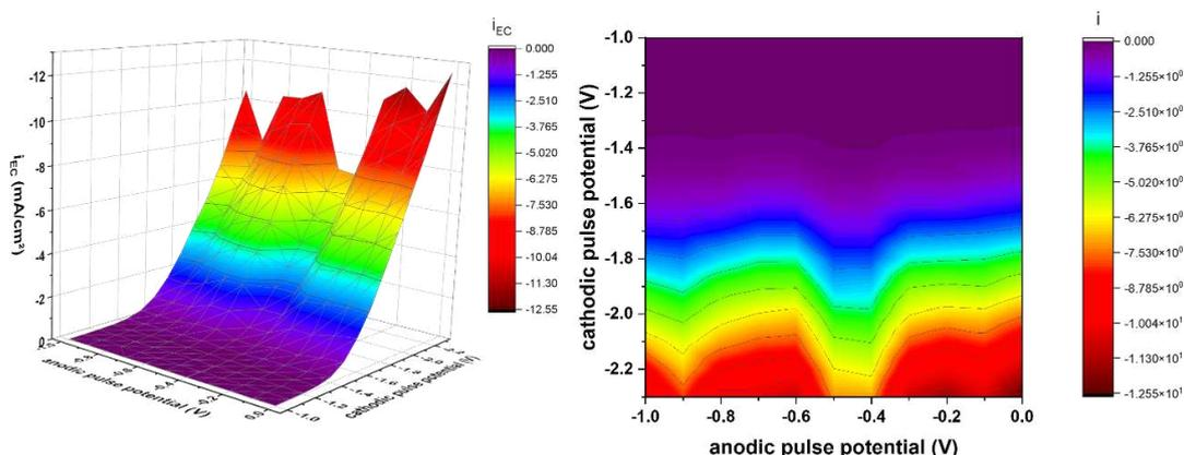
Figure 36: 3D and 2D plot showing the effect of pulse potential variation on  $i_{EC}$ .
