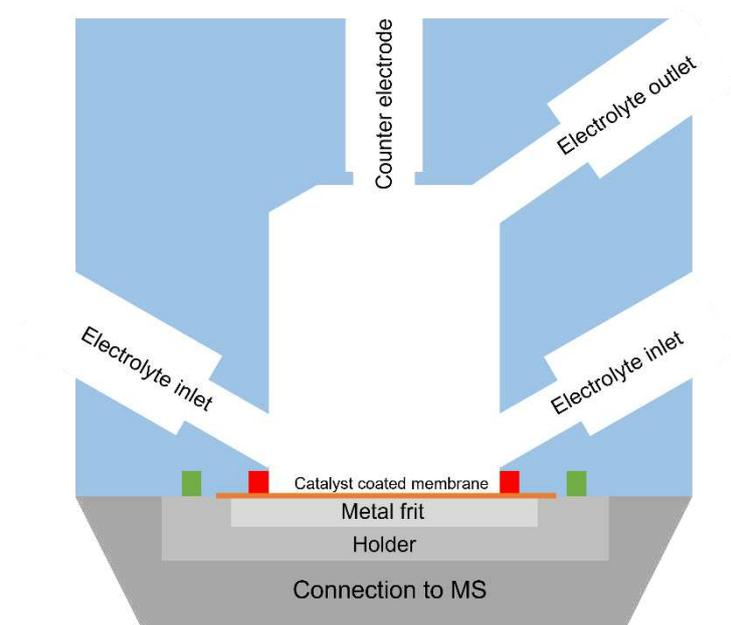
Figure 2: Sketch of the electrochemical DEMS cell used. The orange rectangle represents the catalyst coated membrane, the red and green squares represent individual O-rings of different sizes.
