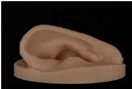
Figure 8 A prosthesis patterns printed directly from silicone using the drop-on-demand technique
