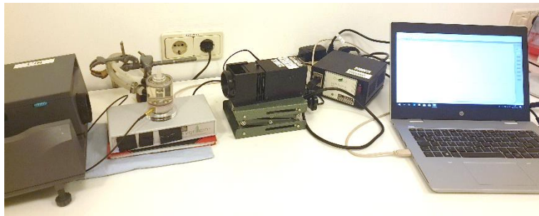
Figure 2.3 - PSII oxygen evolution activity determination set-up (Clark-type electrode). On the table the Hansatech Oxygraph+ with the thermostatic jacket, that includes the sample chamber, can be seen between the two light sources. On the right a control laptop with the O2 view software is displayed.
