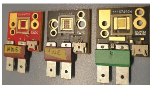
Figure 2.9 – High performance LEDs from Luminus. Red on the left, far red in the middle and green on the right side.
