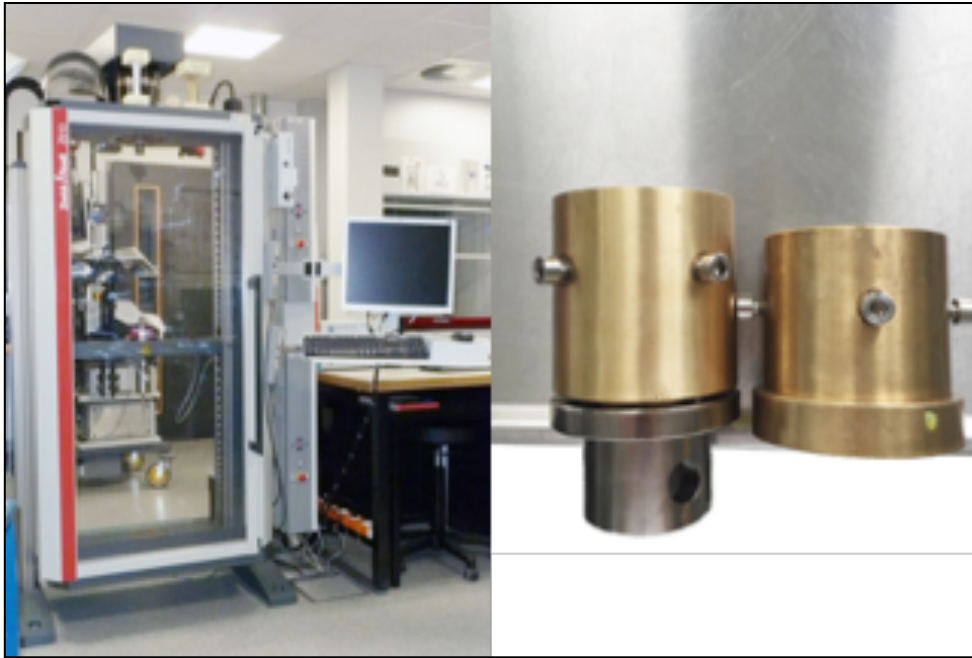
Figure 3. (A) Zwick/Roell 1455 test machine and (B) custom fixation containers.
