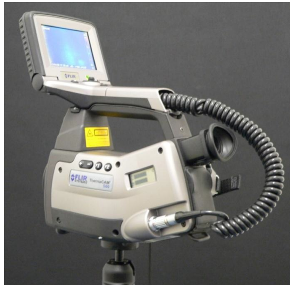
Abbildung 11: ThermaCAM S60 (FLIR Systems GmbH, Frankfurt/Main) [65]
