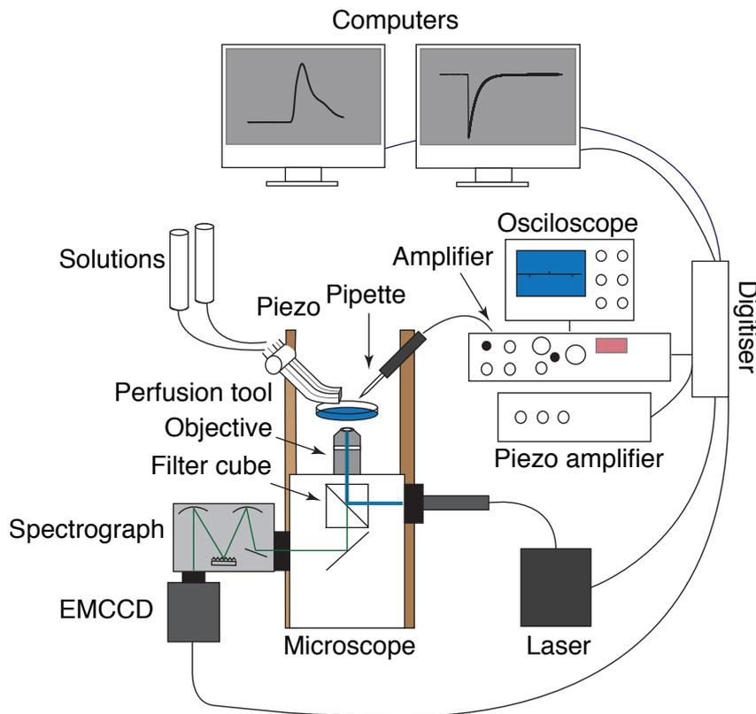
**Figure 6 Experimental setup** A schematic representation of the patch clamp fluorometry setup used for simultaneous acquisition of fluorescence and electrophysiological recordings.
