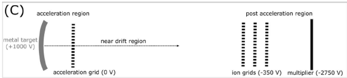
Fig. 18: Scheme of the Chemical Analyzer (CA), its parts and the attached voltages. The metal target is made of Rhodium. Adapted from Klenner et al. 2019
