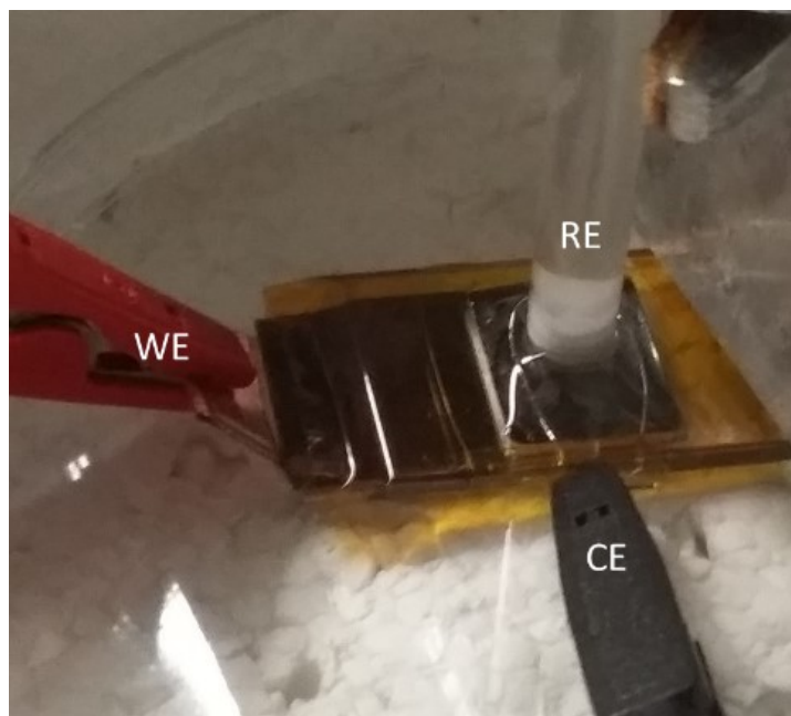
Figure 6.20: Single-time use electrochemical cell for freeze-quench sample preparation, prior to X-ray absorption measurements. The counter electrode is a Pt wire positioned at a distance of 1 mm from the working electrode (X-ray transparent GC). The reference electrode is a \text{Hg}/\text{Hg}_2\text{SO}_4 (saturated), that is removed before freezing the sample.
