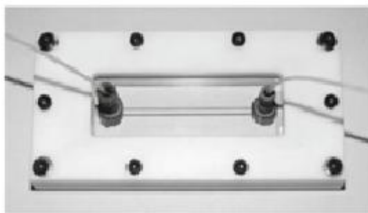
Figure 6.4. Quartz glass microreactor with a single microchannel filled with methylene blue solution. Adapted with permission [11]
