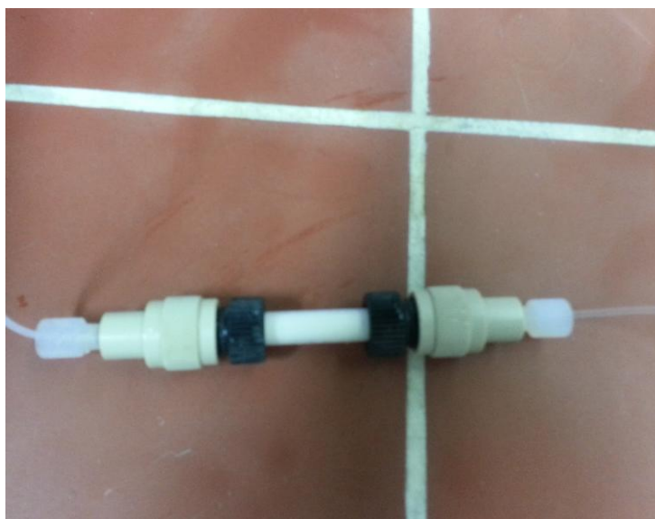
Figure 6.16 Column for enzymatic transformation
