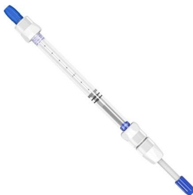
Scheme 6.13. Commercially available Omnifit cartridge. Aadapted with permission. [42]
