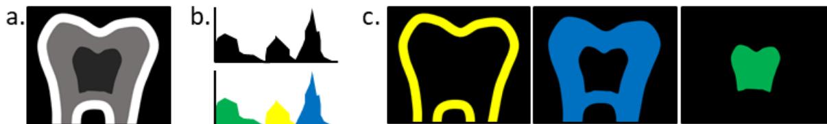
Figure 8: Schematic representation of image segmentation. 3D reconstructed data volumes from PCE-CT are composed of grayscale images (a). The gray values can be compiled and visualized in the form of a histogram (b). The different gray values represent different components of the original image and can be segmented by threshold (c) of the histogram (histogram cropping).
