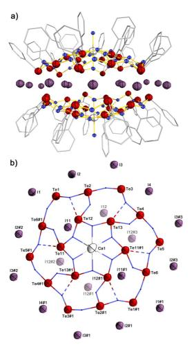
**Figure 4.** a) Structure of **2** and b) top-view to one  $\{(PhTe)_{18}\{Ca-(H_2O)_2\}O_{24}\}^{8+}$  half-shell with the central layer of iodine atoms (the atom 112 and its symmetry related positions possess an occupancy of 0.5.).<sup>[36]</sup>
