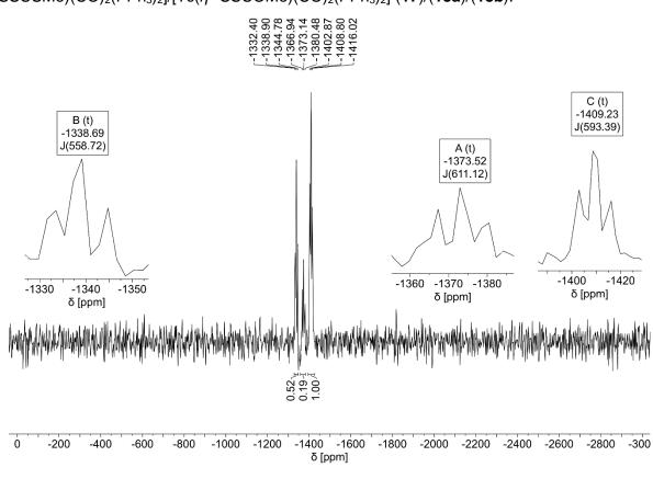
**Figure S65.** <sup>99</sup>Tc NMR spectrum of  $[Tc(\eta^2-SSCMe)(CO)_2(PPh_3)_2]/[Tc(\eta^2-SSCSMe)(CO)_2(PPh_3)_2]/[Tc(\eta^2-SSCOMe)(CO)_2(PPh_3)_2]$  (**17**)/(**18a**)/(**18b**).
