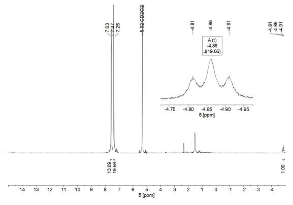
Figure S30. <sup>1</sup>H{<sup>31</sup>P} NMR spectrum of [TcH(CO)<sub>3</sub>(PPh<sub>3</sub>)<sub>2</sub>].
