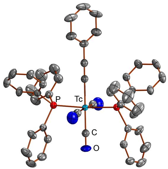
**Figure S7.** Ellipsoid representation (50% probability) of  $[Tc(CCPh)(CO)_3(PPh_3)_2]$  (8a). Hydrogen atoms are omitted for clarity.
