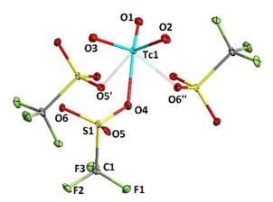
*Figure 2.* ORTEP representation of the coordination of [TcO<sub>3</sub>(OTf)]. Ellipsoids are drawn at the 50% probability level. Selected bond lengths [Å] and angles [°]: Tc1–O1 1.690(3), Tc1–O2 1.683(2), Tc1–O3 1.682(3), Tc1–O4 2.221(3), Tc1–O5' 2.272(2) Tc1–O6" 2.275(2); O1-Tc1-O4 155.4(1), O1-Tc1-O2 105.5(1), O1-Tc1-O3 104.5(1), O1-Tc1-O5' 86.7(1), O1-Tc1-O6" 88.0(1), O4-Tc1-O2 89.9(1), O4-Tc1-O3 89.4(1), O4-Tc1-O5 73.20(9), O5'-Tc1-O6" 73.78(8).
