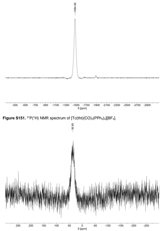
Figure S152. <sup>19</sup>F NMR spectrum of [Tc(tht)(CO)<sub>3</sub>(PPh<sub>3</sub>)<sub>2</sub>][BF<sub>4</sub>].
