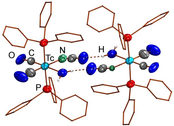
**Figure S3.** Ellipsoid representation (50% probability) of  $[Tc(N_3)(CO)_3(PPh_3)_2]$  (5). Hydrogen atoms are omitted for clarity. The azido ligand is disordered with one of the carbonyl ligands. The major component of the disorder accounts for ca. 70% occupancy.
