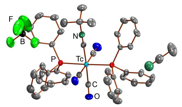
**Figure S15.** Ellipsoid representation (50% probability) of  $[Tc(NCPh)(CO)_3(PPh_3)_2](BF_4)$  (**10a**)  $\cdot CH_2Cl_2$ . Hydrogen atoms are omitted for clarity. The BF<sub>4</sub><sup>-</sup> anion is disordered over two positions in a ratio of ca. 60:40 and was modelled using appropriate constraints and restraints.
