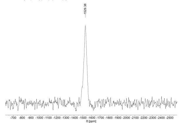
**Figure S40.** <sup>31</sup>P{<sup>1</sup>H} NMR spectrum of [Tc(SeCN)(CO)<sub>3</sub>(PPh<sub>3</sub>)<sub>2</sub>]/[Tc(NCSe)(CO)<sub>3</sub>(PPh<sub>3</sub>)<sub>2</sub>] (8a)/(8b).
