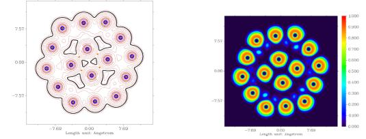
**Fig. S17.** Mapping of the Laplacian of the ED in [{(PhTe)<sub>18</sub>{Ca(H<sub>2</sub>O)<sub>2</sub>}O<sub>24</sub>}<sub>2</sub>l<sub>16</sub>] (**2**) (left: positive = red, negative = blue) and the ELF (right). Positive Laplacian values correspond to local charge depletion, negative values indicate local charge accumulation (areas, where the ED resides).
