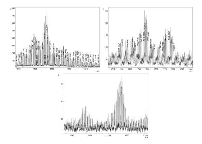
**Figure S103.** Predicted (down) vs. experimental (up) isotope patterns of main species in the ESI<sup>-</sup> mass spectrum of [Ni- $\mu_2$ - $\kappa_2$ -(Ni{ $\kappa_5$ -L<sup>Te</sup>}<sub>2</sub>)<sub>2</sub>- $\mu_2$ -(OAc)<sub>2</sub>]. For the assignments see Figure S95 on page S50.
