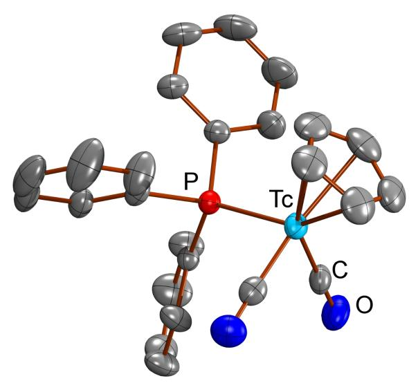
**Figure S3.** Ellipsoid representation (50% probability) of  $[Tc(cp)(CO)_2(PPh_3)]$  (5). Hydrogen atoms are omitted for clarity.
