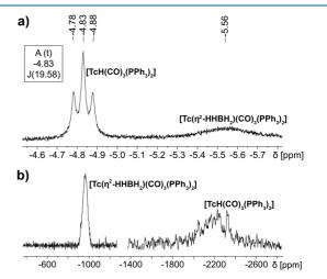
Figure 10. (a)  ${}^{1}$ H and b)  ${}^{99}$ Tc NMR spectra of a mixture of compounds 14 and 15. Note that the  ${}^{99}$ Tc spectrum had to be measured in two windows.
