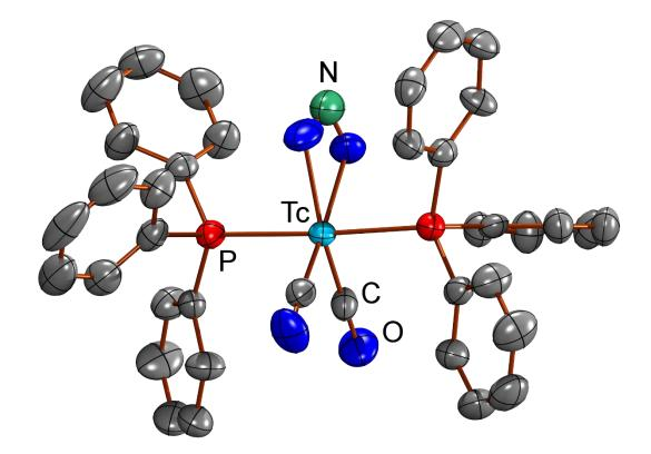
**Figure S10.** Ellipsoid representation (50% probability) of  $[Tc(\eta^1-ONO)(CO)_3(PPh_3)_2]/[Tc(\eta^1-NO_2)(CO)_3(PPh_3)_2]$  (**11a/11b**). Hydrogen atoms are omitted for clarity. The nitrito and nitro isomers of the compound are disordered over the same position with a ratio of 60:40 in favor of the nitrito complex **11a**. The angular distance in the minor nitro isomer was restraint to 2.0 Å and the N-O distances in the nitro isomer were restrained to be similar.
