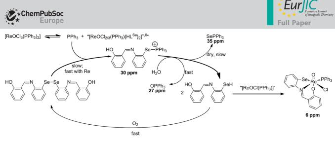
Scheme 2. Proposed mechanism for the reaction between [ReOCl<sub>3</sub>(PPh<sub>3</sub>)<sub>2</sub>] and {HLSe}<sub>2</sub> in CH<sub>2</sub>Cl<sub>2</sub>. Chemical shifts refer to <sup>31</sup>P.
