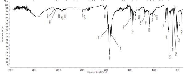
Figure S63. IR spectrum of  $[TcH(CO)_3(PPh_3)_2]/[Tc(\eta^2-HHBH_2)(CO)_2(PPh_3)_2]$  (14)/(15).
