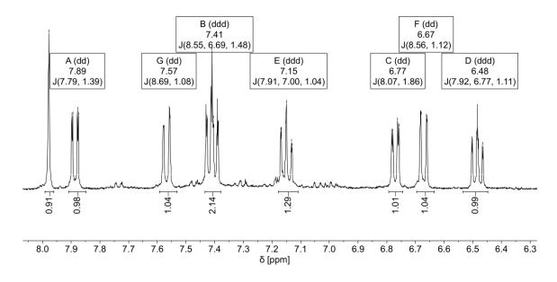
**Figure S10.** <sup>1</sup>H,<sup>1</sup>H-COSY NMR spectrum of  $[Pd_4(L'^{Se})_4]$  in  $CD_2Cl_2$  focused on the aromatic region.
