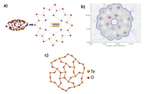
**Fig. S12.** (a) Scheme of the tellurium-iodine interactions, according to the topological analysis, (b) Electron density map of the plane formed by the iodine atoms, (c) Scheme of the Te-O half-shell according to the topological analysis.
