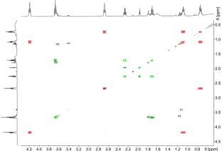
Figure 3.  ${}^{1}H_{1}H$ -COSY NMR spectrum of a mixture of [Tc-(=*cyclo*-C(CH<sub>2</sub>)<sub>4</sub>O)(CO)<sub>3</sub>(PPh<sub>3</sub>)<sub>2</sub>](BF<sub>4</sub>) (red) and 1-pentyne-5-ol (green).
