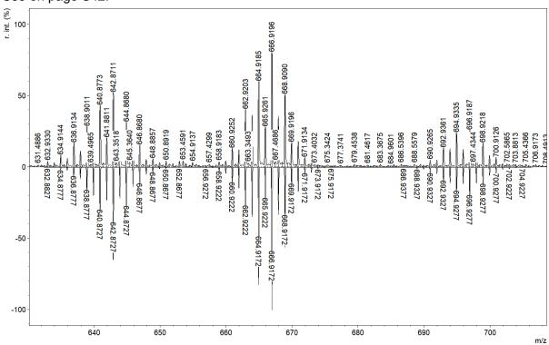
**Figure S77.** Predicted (down) vs. experimental (up) isotope patterns of main species in the ESI<sup>-</sup> mass spectrum of [Ni- $\mu_2$ - $\kappa_2$ -(Ni{ $\kappa_5$ -L<sup>Se</sup>}\_2)<sub>2</sub>- $\mu_2$ -(OAc)<sub>2</sub>]. For the assignments see Figure S69 on page S42.
