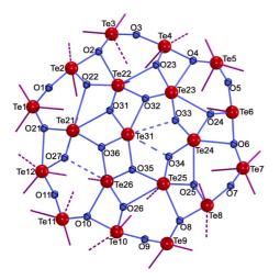
**Figure 3.** Te–O network of **1 b** with designation of Te–I interactions with the central layer of iodine atoms. Dotted lines indicate Te–O (blue) and TeI (purple) interactions larger than 3.220 Å and 3.636 Å, respectively (90% of the sum of the van der Waals radii). Solid lines represent shorter bonds.<sup>[36]</sup>
