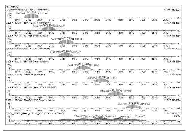
Fig. S5. Triply charged ions of compound 1b (simulations: top rows, experimental: bottom row).
