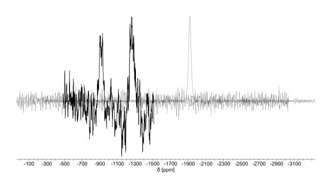
**Figure S195.** <sup>99</sup>Tc NMR spectrum (overlay between all relevant spectral regions) for the reaction between  $[TcH(CO)_3(PPh_3)_2]$  and  $[H(OEt_2)_2][BArF_{24}]$  in dry, degassed  $CD_2Cl_2$  under Ar; addition of solvent performed at 100 K. Time: 3 d.
