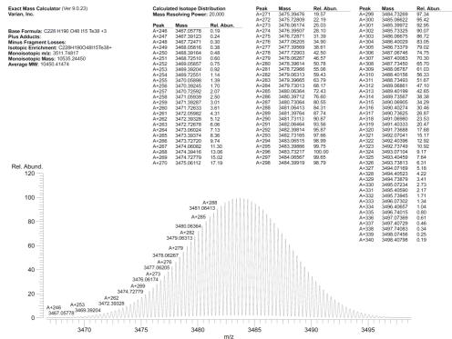
**Fig. S1.** Simulation of the  $[M-3I]^{3+}$  of compound **1b**,  $[\{(PhTe)_{19}O_{24}\}_{2}I_{18}]$ , using the "Exact Mass Calculator", showing the capability of the software to depict a wider isotopic pattern as well as to simulate at different theoretical resolutions. For data analysis, we set the resolution to 30,000 as default.
