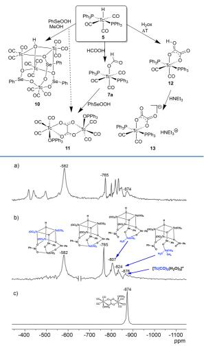
Figure 8. <sup>99</sup>Tc NMR spectra of (a) a  $CH_2Cl_2$  extract of the crude residue obtained from a reaction between 5 and PhSeOOH in toluene/MeOH/H<sub>2</sub>O, (b) a solution of 10 in (moist)  $CH_2Cl_2$ , and (c) a solution of 11 in  $CH_2Cl_2$ .
