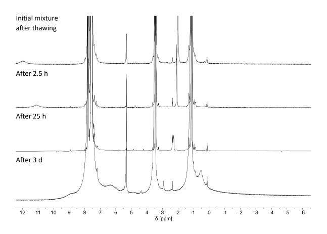
**Figure S198.** <sup>1</sup>H NMR spectra (stacked) for the reaction between  $[TcH(CO)_3(PPh_3)_2]$  and  $[H(OEt_2)_2][BArF_{24}]$  in dry, degassed thf-d8 under Ar; addition of solvent performed at 100 K.
