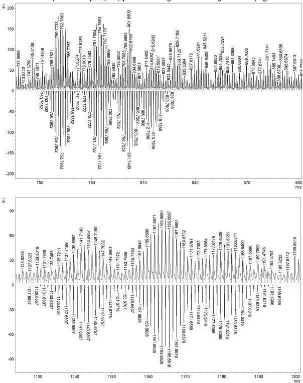
**Figures S30-S34.** Predicted (down) vs. experimental (up) isotope patterns of main species in the ESI<sup>+</sup> mass spectrum of  $[Pd_4(L'^{Se})_4]$ . For the assignments see Figure 22 on page S25.
