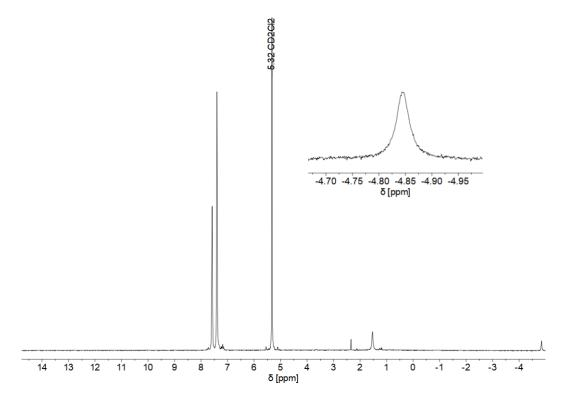
Figure S31. <sup>99</sup>Tc NMR spectrum of [TcH(CO)<sub>3</sub>(PPh<sub>3</sub>)<sub>2</sub>].
