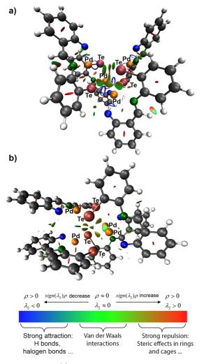
**Figure 4.** RDG plots (a) of the gas-phase structure of the cuboid-like  $[Pd_4(L'^{Te})_4]$  cluster at an isodensity of 0.3 with a grid spacing of 0.05 bohr and (b) of the  $CH_2Cl_2$  solution structure of the gyrobifastigial  $[Pd_4(L'^{Te})_4]$  at an isodensity of 0.20 with a grid spacing of 0.05 bohr.
