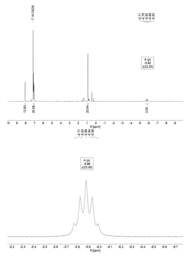
Figure S27. <sup>99</sup>Tc NMR spectrum of [TcH<sub>3</sub>(PPh<sub>3</sub>)<sub>2</sub>(PMe<sub>3</sub>)<sub>2</sub>].
