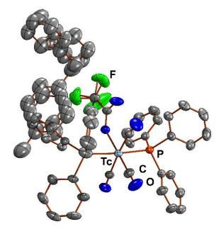
**Figure S6.** Ellipsoid representation (50% probability) of  $[Tc(\eta^1-O(CH)O)(CO)_3(PPh_3)_2] \cdot 0.5$  toluene. Hydrogen atoms are omitted for clarity.
