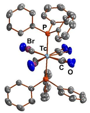
**Figure S4.** Ellipsoid representation (50% probability) of the structure of  $[Tcl(CO)_3(PPh_3)_2]$ . Hydrogen atoms are omitted for clarity.
