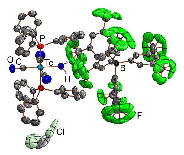
**Figure S2.** Ellipsoid representation (50% probability) of  $\alpha$ -[Tc(OH<sub>2</sub>)(CO)<sub>3</sub>(PPh<sub>3</sub>)<sub>2</sub>][BF<sub>4</sub>] (**1b**). Hydrogen atoms bonded to carbon atoms are omitted for clarity. The water hydrogen atoms were located in the density map and refined freely.
