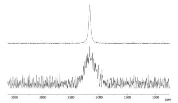
Figure 5. <sup>99</sup>Tc NMR spectra of a) compound 2 and b) compound 4 in  $CH_2Cl_2$  with a strong line broadening for 4 indicating a dynamic behavior in solution.
