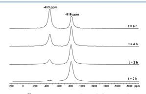
Figure 3.  $^{99}$ Tc NMR spectra obtained from a solution of  $[Tc(NO)(SCN)(Cp)(PPh_3)]$  in boiling toluene.
