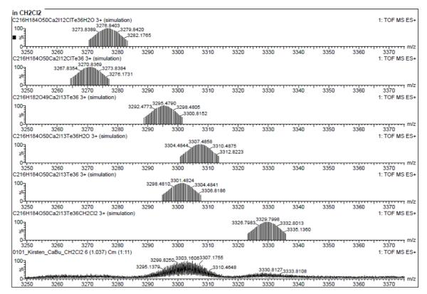
Fig. S8. Region of triply charged ions in the (+)-ESI MS pf compound 2, top rows: simulations, bottom row: experimental data.
