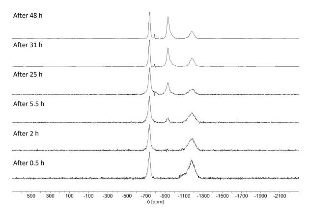
**Figure S203.** *In-situ* NMR spectrum of the reaction between  $[Tc(OH_2)(CO)_3(PPh_3)_2]^+$  and DMSO. Stacking of <sup>99</sup>Tc-spectra focussed on the region around -1000 ppm.
