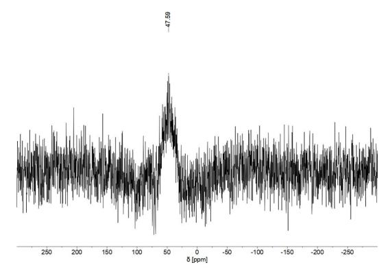
Figure S63. <sup>99</sup>Tc NMR spectrum of  $[Tc(\eta^2-OO(CPh))(CO)_2(PPh_3)_2]$ .
