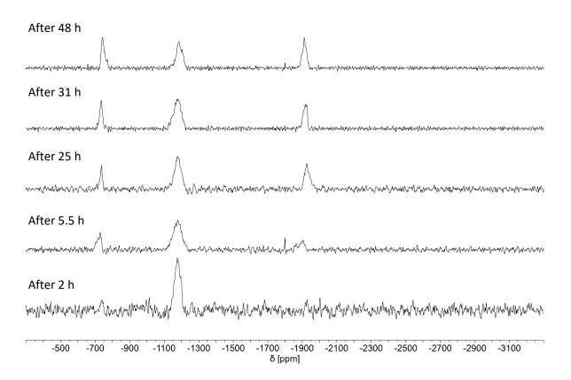
**Figure S206.** *In-situ* NMR spectra of the reaction between  $[Tc(OH_2)(CO)_3(PPh_3)_2]^+$  and bpy without the addition of a base. Stacking of <sup>99</sup>Tc-spectra.
