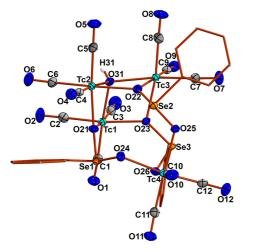
Figure 9. Molecular structure of  $[{Tc(CO)_3}_3(\mu^3-OH)(\mu^2-O(SePh)-O)_3{Tc(CO)_3}]$  (10). Ellipsoids are depicted at 50% probability. Phenyl hydrogen atoms and further labels are omitted for clarity.
