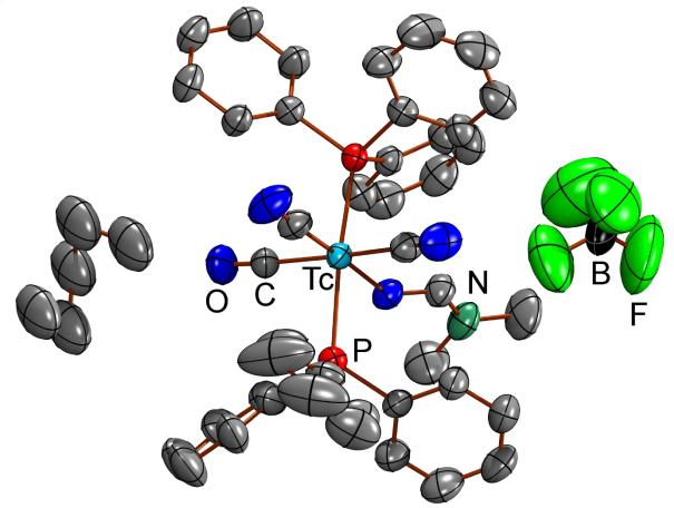
**Figure S8.** Ellipsoid representation (50% probability) of  $[Tc(DMF)(CO)_3(PPh_3)_2][BF_4]$  (4). Hydrogen atoms are omitted for clarity. The  $[BF_4]^-$  counter-ion is somewhat ill-defined and modelled using appropriate constraints and restraints. The crystal was treated as a three-component twin. The overall quality of this structure is low. Restraints were mainly used to improve the thermal motion of the BF<sub>4</sub> anion.
