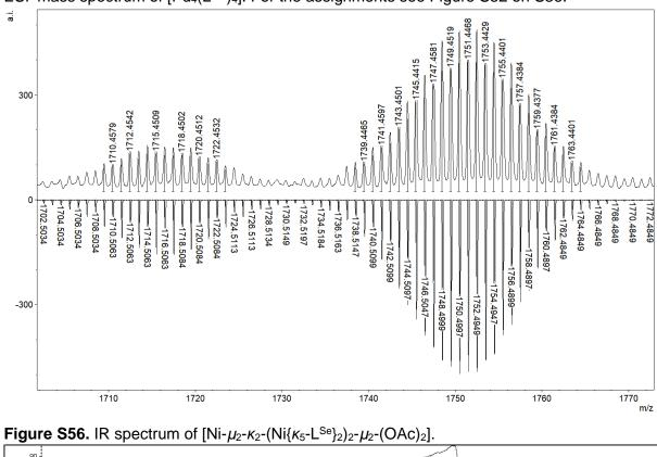
**Figure S55.** Predicted (down) vs. experimental (up) isotope patterns of main species in the ESI<sup>-</sup> mass spectrum of  $[Pd_4(L'^{Te})_4]$ . For the assignments see Figure S52 on S36.
