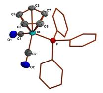
**Figure 2**. a) Solid-state structure of  $[Tc(Cp)(CO)_2(PPh_3)_2]$  (5) (Tc-C1 1.881(2), Tc-C2 1.890(2), Tc-C3 2.307(2), Tc-C4 2.282(2), Tc-C5 2.283(2), Tc-C6 2.306(2), Tc-C7 2.308(2), Tc-C<sub>centroid</sub> 1.959(1) Å).
