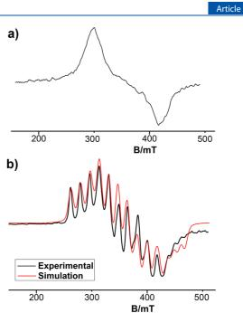
**Figure 5.** X-band EPR spectra of  $[Tc(NO)(I)_2(Cp)]$  in CHCl<sub>3</sub> (a) at room temperature and (b) at T = 77 K.
