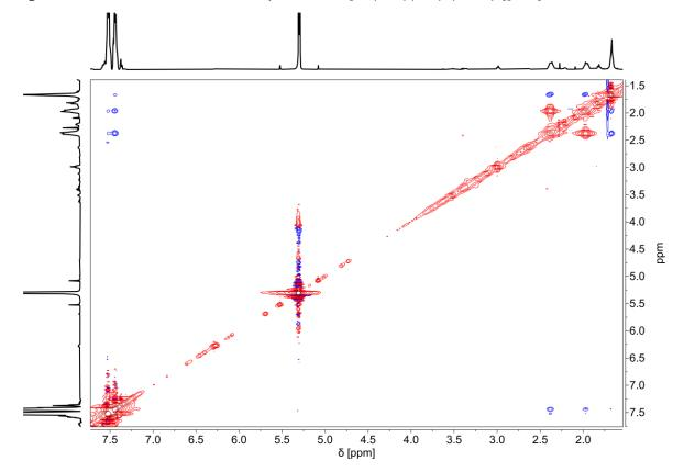
Figure S174. <sup>1</sup>H,<sup>1</sup>H-NOESY NMR spectrum of [Tc(thte)(CO)<sub>3</sub>(PPh<sub>3</sub>)<sub>2</sub>][BF<sub>4</sub>].
