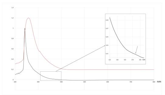
**Fig. S21.** Experimental UV/Vis spectra of [{(PhTe)<sub>19</sub>O<sub>24</sub>}<sub>2</sub>]<sub>18</sub>] (**1b**) (red) and [{(PhTe)<sub>18</sub>{Ca(H<sub>2</sub>O)<sub>2</sub>}O<sub>24</sub>}<sub>2</sub>]<sub>16</sub>] (**2**) (black). Note the shoulder at approximately 380 nm, which corresponds to the calculated value (Fig. S13b). The corresponding band in the spectrum of **1b** is not resolved.
