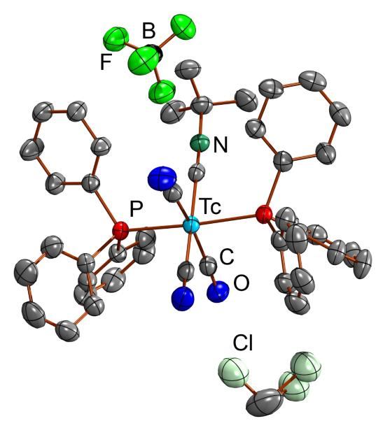
**Figure S14.** Ellipsoid representation (50% probability) of  $[Tc(CN'Bu)(CO)_3(PPh_3)_2](BF_4)$  (**9b**)  $\cdot$  CH<sub>3</sub>CN. Hydrogen atoms are omitted for clarity.
