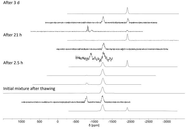
**Figure S196.** <sup>99</sup>Tc NMR spectra (stacked) for the reaction between  $[TcH(CO)_3(PPh_3)_2]$  and  $[H(OEt_2)_2][BArF_{24}]$  in dry, degassed  $CD_2Cl_2$  under Ar; addition of solvent performed at 100 K.
