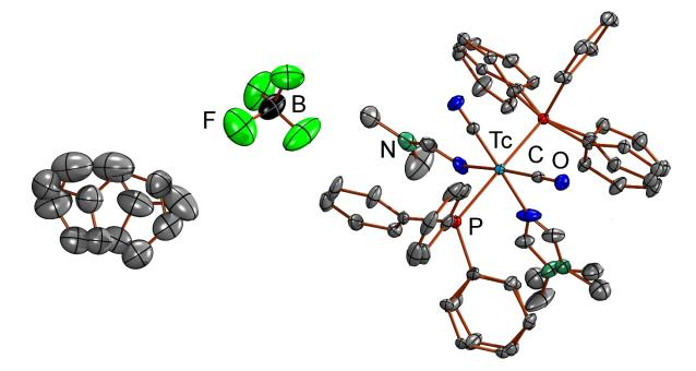
**Figure S10.** Ellipsoid representation (50% probability) of  $[Tc(CO)_4(PPh_3)_2][BArF_{24}]$  (**6a**)  $\cdot$  0.25CH<sub>2</sub>Cl<sub>2</sub>. Hydrogen atoms are omitted for clarity. Most of the CF<sub>3</sub>-groups are expectedly disordered over two positions. Restraints were mainly used to model the disordered CF<sub>3</sub> groups.
