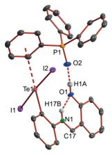
Figure 3. Structure of {[(HO)C<sub>6</sub>H<sub>4</sub>-(CHN<sup>+</sup>H)-C<sub>6</sub>H<sub>4</sub>-Tel<sub>2</sub>)·OPPh<sub>3</sub>}. Ellipsoids are depicted at 50 % probability. Hydrogen atoms bonded to carbon atoms are omitted for clarity.
