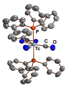
**Figure S10.** Ellipsoid representation (50% probability) of  $[Tc(\eta^2-Et_2btu)(CO)_2(PPh_3)_2]$ . Hydrogen atoms are omitted for clarity.
