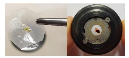
Figure S 1. Pertechnetyl triflate immediately after preparation on Scotch tape (left) and five minutes after inserting into mounting disk (right). Only reflections of NH<sub>4</sub>TcO<sub>4</sub> were observed. The brown material is attributed to TcO<sub>2</sub>.
