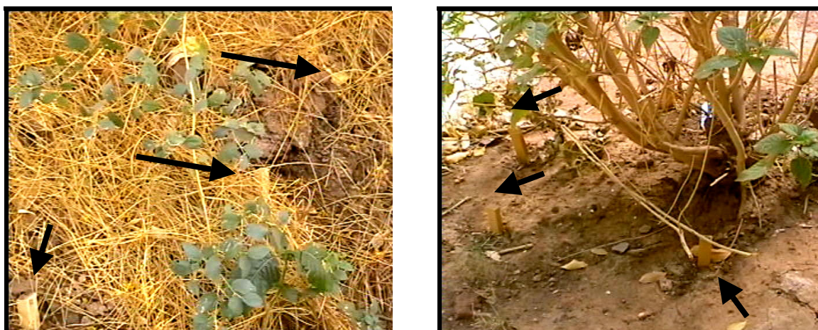
Fig 7: Experimental design with impregnated wooden baits (arrows) in the field.
