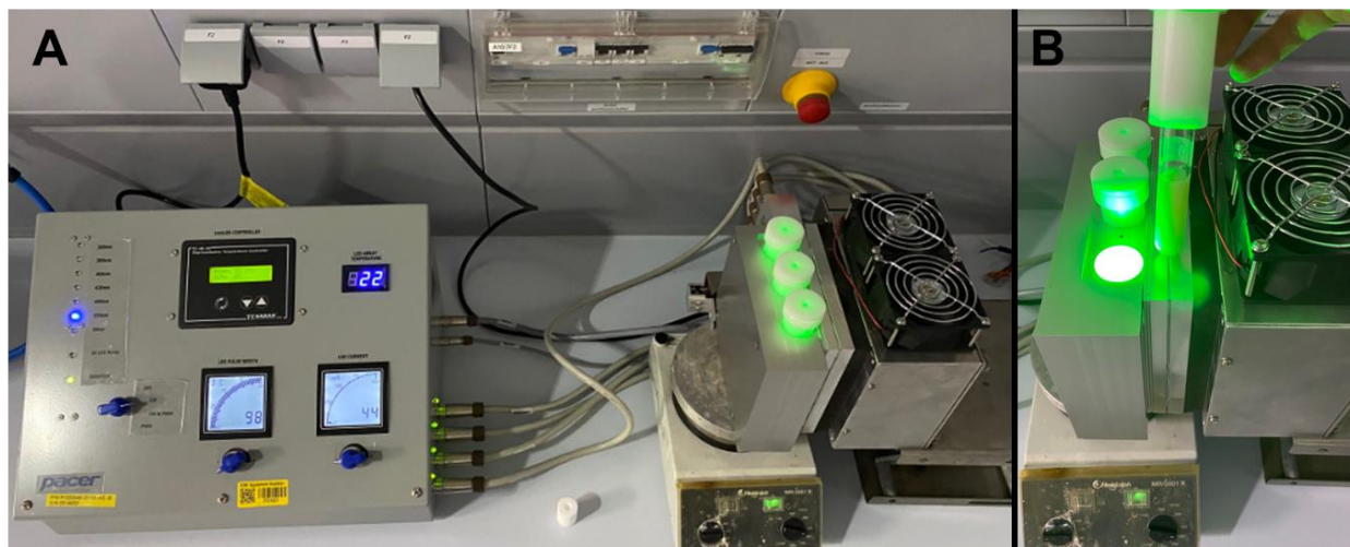
Figure S4.5. Photoreactor used for the CN-OA-m/UPO system; A) Complete photoreactor unit with control panel unit (left) and reactor and cooling unit (right); B) Reactor unit on a magnetic stirrer with microwave reaction vials: The reactor has three slots for microwave reaction vials. A magnetic stirrer is used to stir the reaction (500 rpm). The photoreactor is controlled by a control unit allowing to adjust the temperature, light intensity (25-500 mA), and wavelength. Six different wavelengths can be used for reactions (365 nm, 385 nm, 405 nm, 420 nm, 455 nm and 528 nm).
