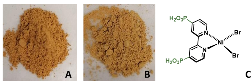
Figure S6.5. Unfunctionalized CN-OA-m (A) and CN-OA-m–NiBr 2 ·dpbpy (Cat 1) (B). Structure of NiBr 2 ·dcbpy (C). The functionalities that bind to the surface of CN-OA-m are marked in green.
