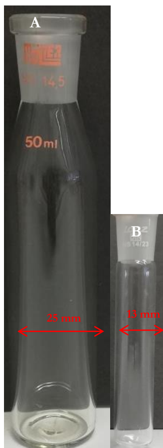
Figure S3.11. Vessel dimensions of vial for scale-up reaction (A) and vial for “standard scale” reactions (B).
