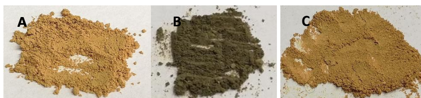
Figure S3.9. Fresh CN-OA-m (A), CN-OA-m after recyclability tests with white light irradiation (B) and CN-OA-m after recyclability tests with green light irradiation (C).
