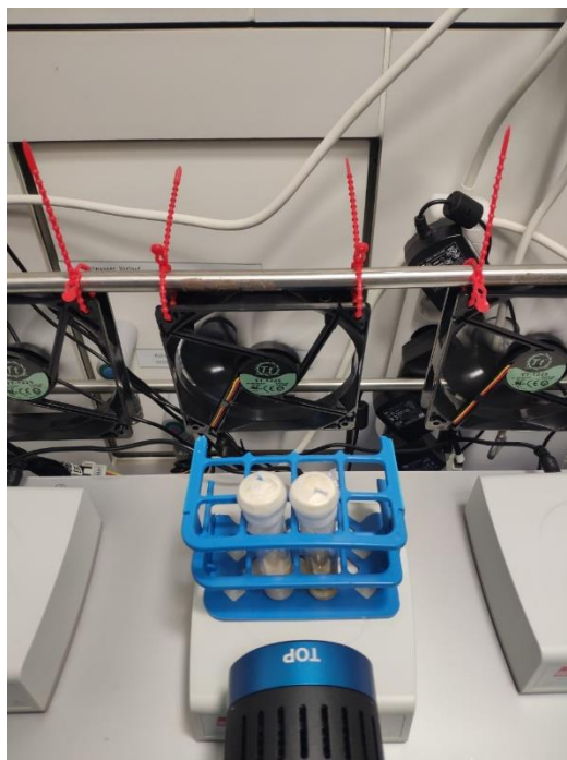
Figure S7.19. Image of the setup using a single blue LED lamp.
