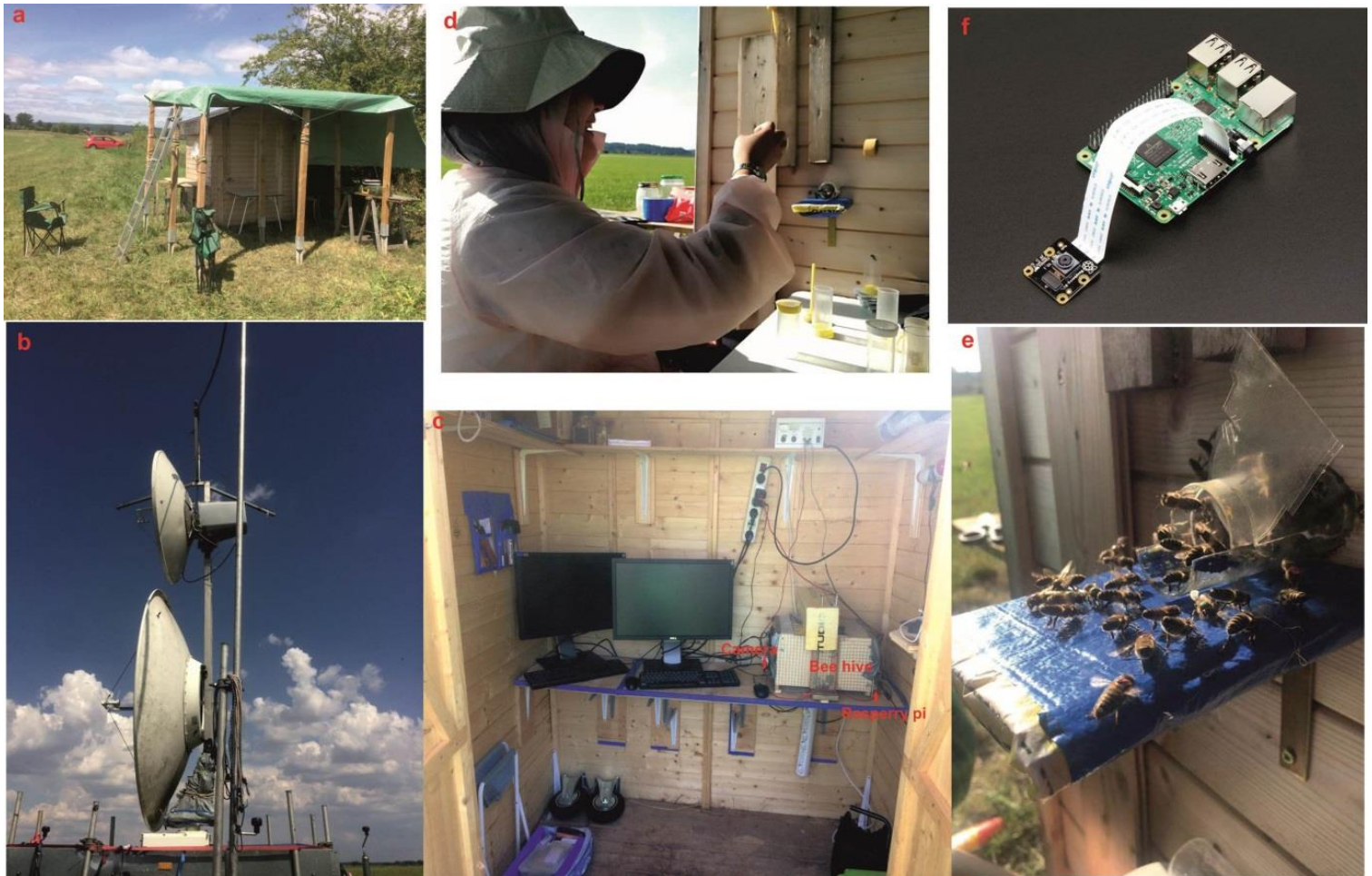
Figure 18. Experimental setup. 'a', cabin for the bee colony; 'b', harmonic radar; 'c', bee colony with camera and raspberry pi; 'd', experimental observer capturing bees at one side of exit; e, bees fanning at the hive exit; d, raspberry pi with camera.
