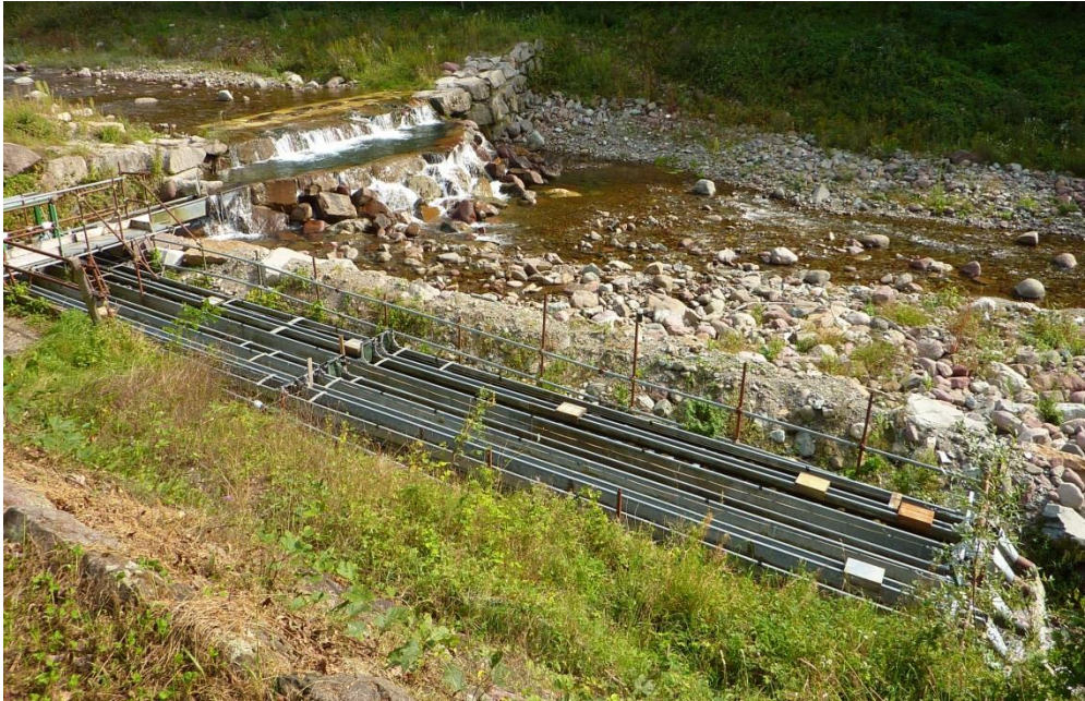
Figure 3. Side view of the stream-side experimental flume system on the Fersina stream (Trentino Province, NE Italy). Flow runs from left to right. Photo: M. Grubisic.
