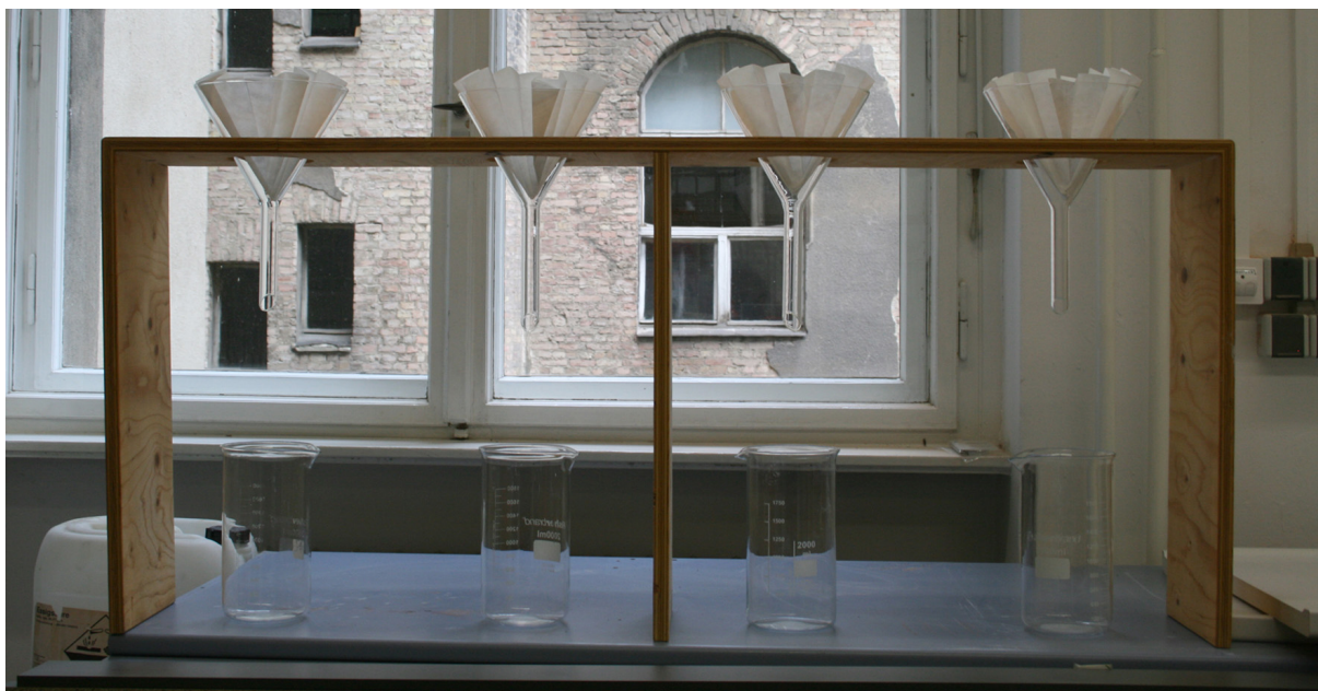
Figure 8 Fluted filters for extracting the coarse sample fraction from the sediment NaCl or HCl slush. The set-up was designed to process four samples at once.
