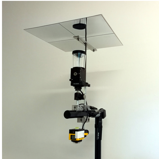
Figure 3.7: Omnidirectional cameras mounted on the ROSStuhl. The one above is the LoReNav camera, a catadioptric camera with a hyperbolic mirror. The sun cover reduces direct exposure to the sunlight. Its lower side is covered with mirrors to prevent biasing the exposure controller. The omnidirectional camera below is a Kodak SP360.
