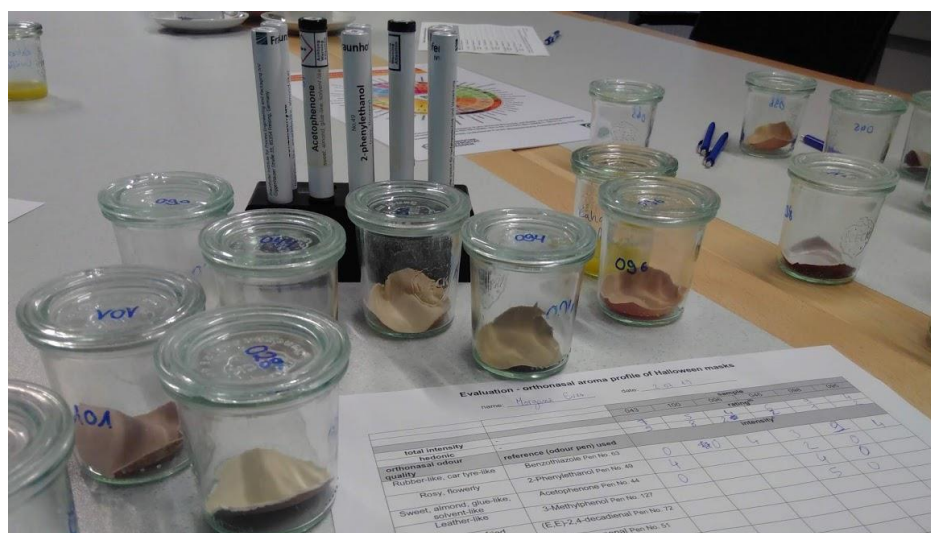
Figure 6: Human sensory evaluation, panelists open the lid and immediately smell the samples to record their odor impressions; odorous pens with standard substances are used to help the rating of single attributes.
