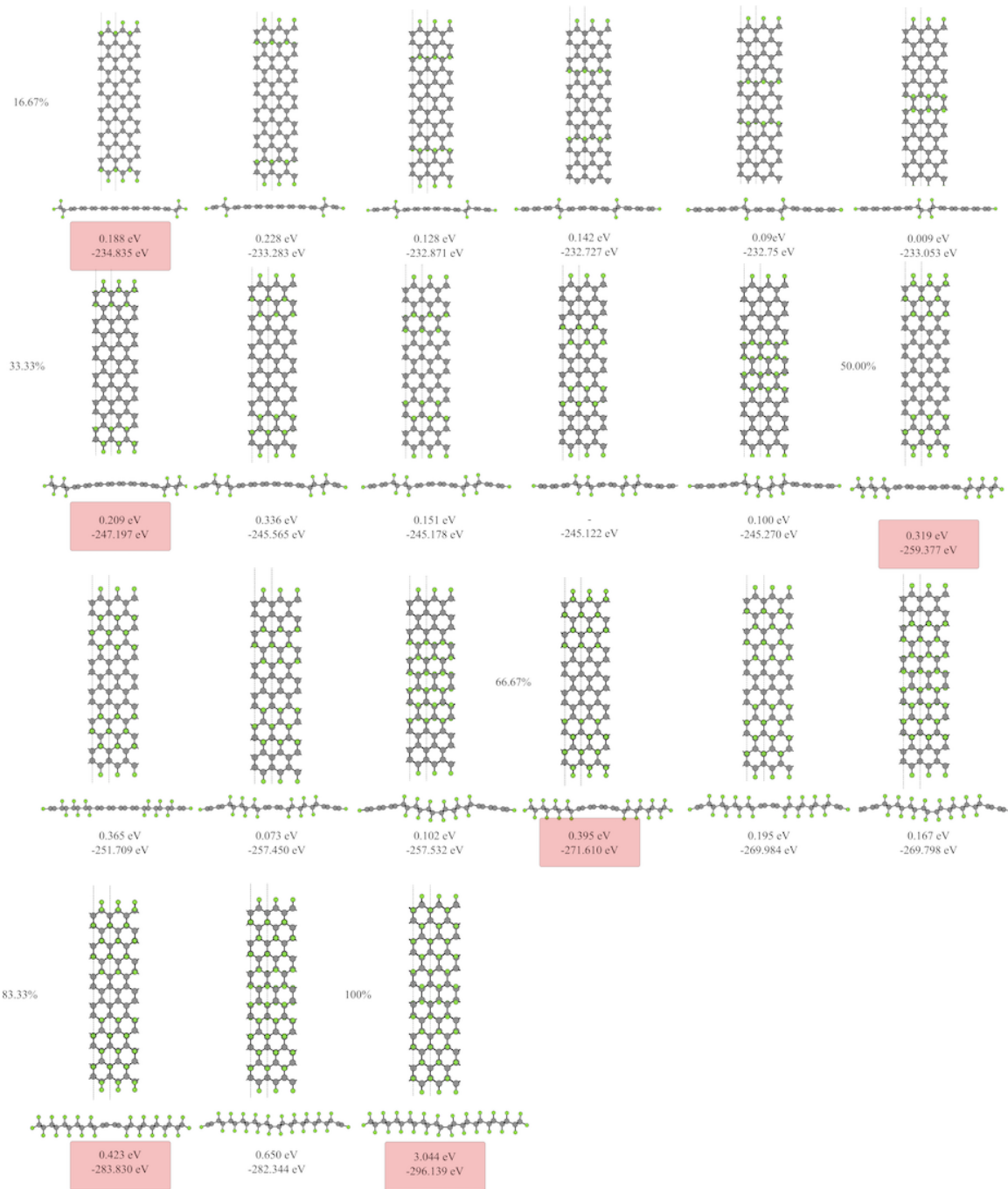
Figure S5: Top and sides views of symmetric fluorinated F-12ZGNRs (PBE optimized structures). The band gap values and the total energy are listed below each structure. The structure within each fluorination degree obtained with the lowest energy is marked in red and is reported in the main text. The xyz coordinates of the optimized structures will be available from the authors upon request.
