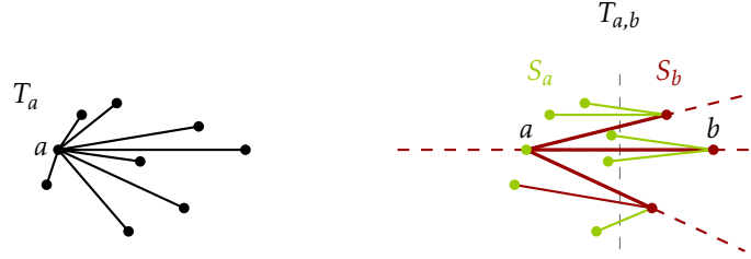
Figure 6.1: A star T_a and a tree T_{a,b} , the rays bounding the cones are drawn dashed.
