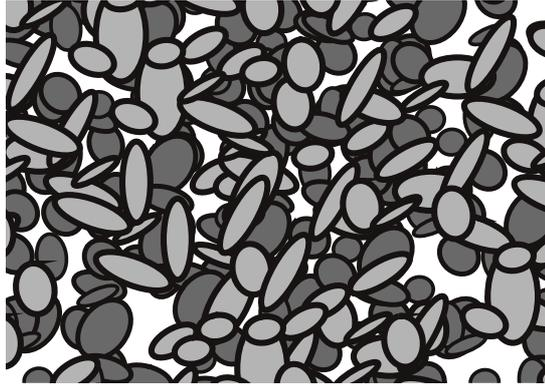
Figure 1.1: Simplified illustration of rocks on the grain scale. The pore space (white) in between the rocks solid constituents (grey) is in-situ filled with fluids (liquid or gaseous).
