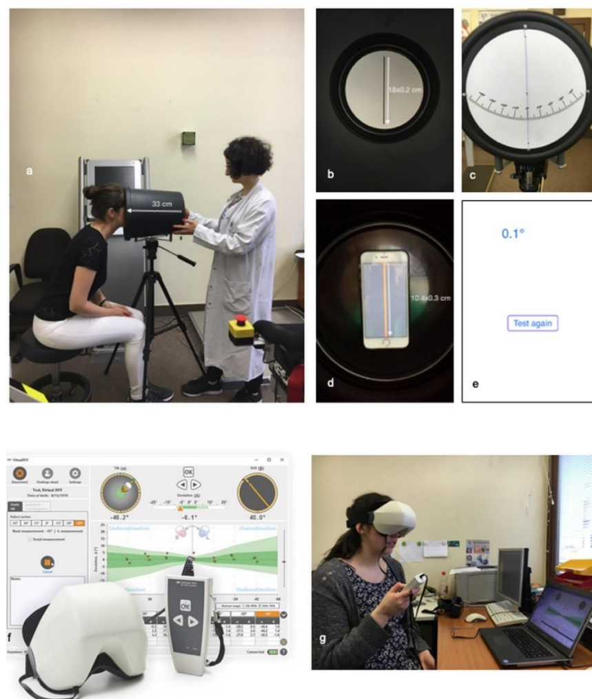
Figure 1. Examination set-up with the analog and digital bucket. (a) Examination of the subjective visual vertical (SVV) with the bucket test (distance from participant’s eyes to line on the bottom of the bucket 33 cm); (b) view of the analog bucket test for a participant (measures of the line: 18 \times 0.2 cm); (c) view of the analog bucket test for an examiner; (d) view of the Visual Vertical app for a participant (measures of the line: 10.4 \times 0.3 cm); (e) result of the Visual Vertical app as seen by the examiner; (f) C-SVV ® goggles (image reproduced with permission from Diatec Diagnostics GmbH and was reused from [13] with permission of Springer); (g) examination of SVV with the C-SVV ® goggles.
