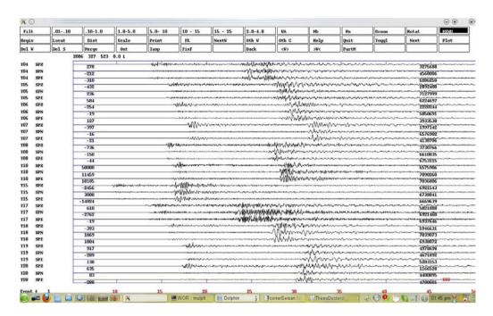
Figure 4.4: An example of a deeper event (53.8 km,  $M_L = 5.5$ ) registered by the WFFS network in 2006.03.27 at the Longitudinal Valley near to the Nazca plate.
