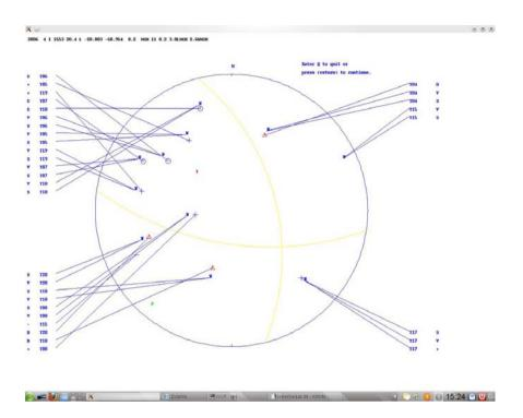
Figure 4.12: An example of calculation of the focal mechanism using SEISAN [Havskov and Ottemöller, 2000]. T indicates T-axis, P indicates P-axis. The circles and + simbols indicate stations with compression in their P-wave arrivals. Triangles and - simbols indicate dilatation in their P-wave arrivals. V indicates amplitude ratio SV/P. S indicates amplitude ratio SV/SH.
