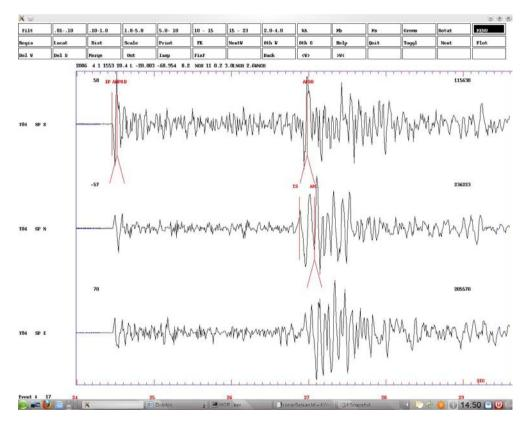
Figure 4.10: An example of hand-picked P and S arrivals for a single station using SEISAN [Havskov and Ottemöller, 2000]. IP means impulsive P, AMPG indicates amplitude for P used in the calculation of SV/P amplitude ratio, D indicates polarity (dilatation), IS indicates impulsive S, AML indicates amplitude for local magnitude, AMSG indicates amplitude for SV used in the calculation of SV/P amplitude ratio.
