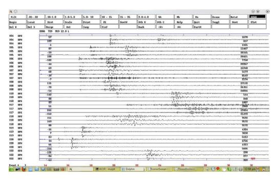
Figure 4.3: An example of a shallow event (1 km,  $M_L = 1.7$ ) registered by the WFFS network in 2006.07.29 at the east flank of the Precordillera.
