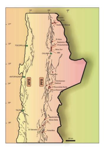
**Figure 2.5:** The two large scale margin-parallel shear zones (after *Camus* [2003]), the Atacama Fault System (AFS) and the Precordillera Fault System (PFS). The red dots indicate the location of the most important Porphyry Cooper deposits in the region, which are shown with their names. All Porphyry Cooper deposits are spatially related to PFS. The green rectangles indicate the cities in the Antofagasta region
