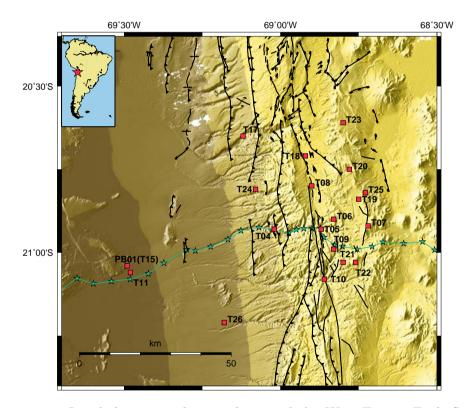
Figure 4.1: Local short period network around the West Fissure Fault System (WFFS). On the map the stations locations are plotted by red squares –the broad band station (PB01) from the IPOC network is in the same place that T15– and WFFS by black lines after *Reutter et al.* [1994], *Camus* [2003], *SERNAGEOMIN* [2003] and *Victor et al.* [2004]. The W-E crooked green line indicates the ANCORP profile with shot points (green stars).
