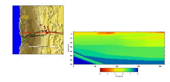
Figure 4.2: The 2-D P-velocity model by  $L\ddot{u}th$  [2000]. On the left: the straight red line indicates the position of the velocity model, the black line and crosses indicate the ANCORP profile, the red squares indicate some short period stations from WFFS network, and the green squares indicate the broad band stations from the IPOC network. On the right: The cross section view of the 2-D P-velocity model, the colors indicate the different velocities (see the colors bar).
