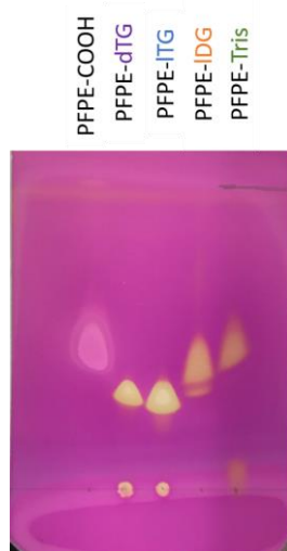
Figure S1. TLC analysis of PFPE-COOH, PFPE-dTG, PFPE-ITG, PFPE-IDG, and PFPE-Tris from left to right, respectively. A mixture of 20% methanol (v/v) and HFE-7100 was used as a mobile phase to run the TLC.
