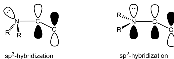
Figure 4: Extreme cases of hybridization at the nitrogen atom and the resulting overlaps with the LUMO of the C-C double bond.
