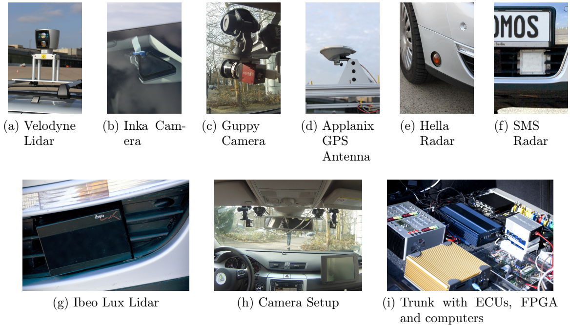
Figure 6.3: Sensor and computing devices close-ups and mounting
