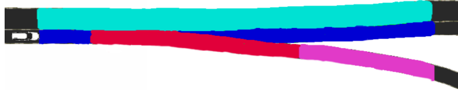
(b) Spatial horizon containing all road segments in front of the vehicle within a given travel distance.
