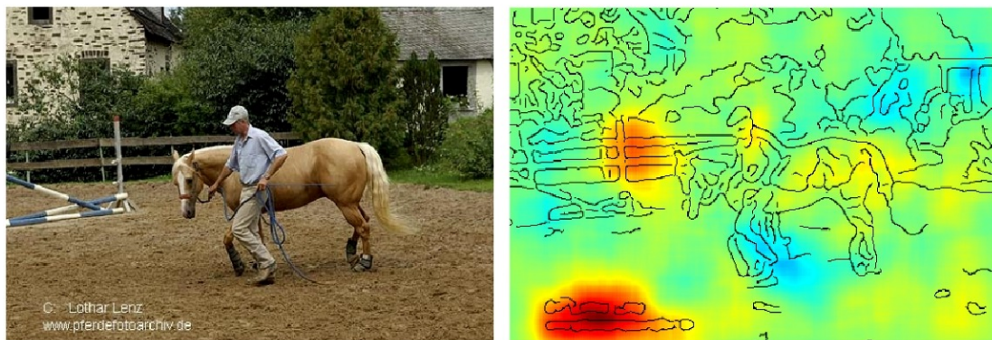
Figure 1.1: Explaining Machine Learning Predictions. A model that correctly classifies the left image as containing a horse is doing so by detecting a small copyright text not being present in other classes. The heat map shows the output of a method called layer-wise relevance propagation that highlights in red color which parts of an image are most relevant for the model prediction. The image is adapted from [2].
