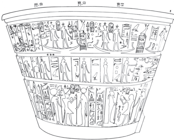
Fig. 5 Sketch of an Egyptian Water clock.
