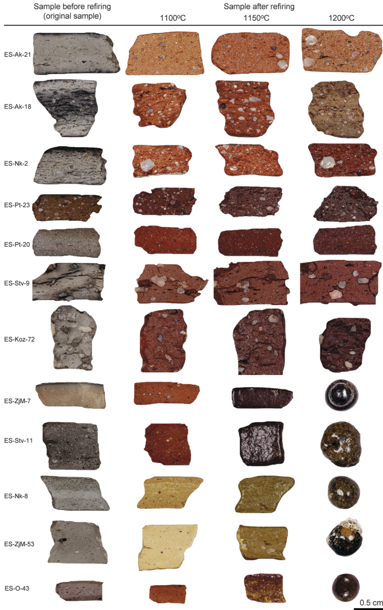
Fig. 15 Examples of various matrix categories and various matrix types. The seven first samples are made of various non-calcareous clays coloured to varying degrees by iron-compounds. Two of the samples (ZjM-7 and Stv-11) are made of non-calcareous clays enriched with carbonates in sub-10 µm fraction. The next two samples are made from calcareous clays. The last sample (O-43) is made of a mixed clay (with a predominance of non-calcareous clay). Samples (cut-sections) before and after refiring in air.
