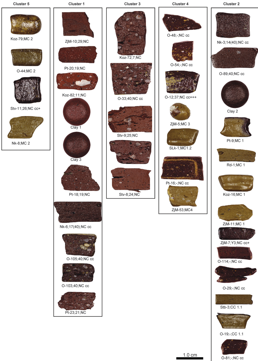
Fig. 22 Samples examined using both MGR-analysis and chemical analysis by WD-XRF. Samples arranged in order determined by cluster analysis, see dendrogram shown in figure 17. Samples (cut-sections) after refiring and three specimens of fired clay samples, refiring/firing at 1150°C in air.
