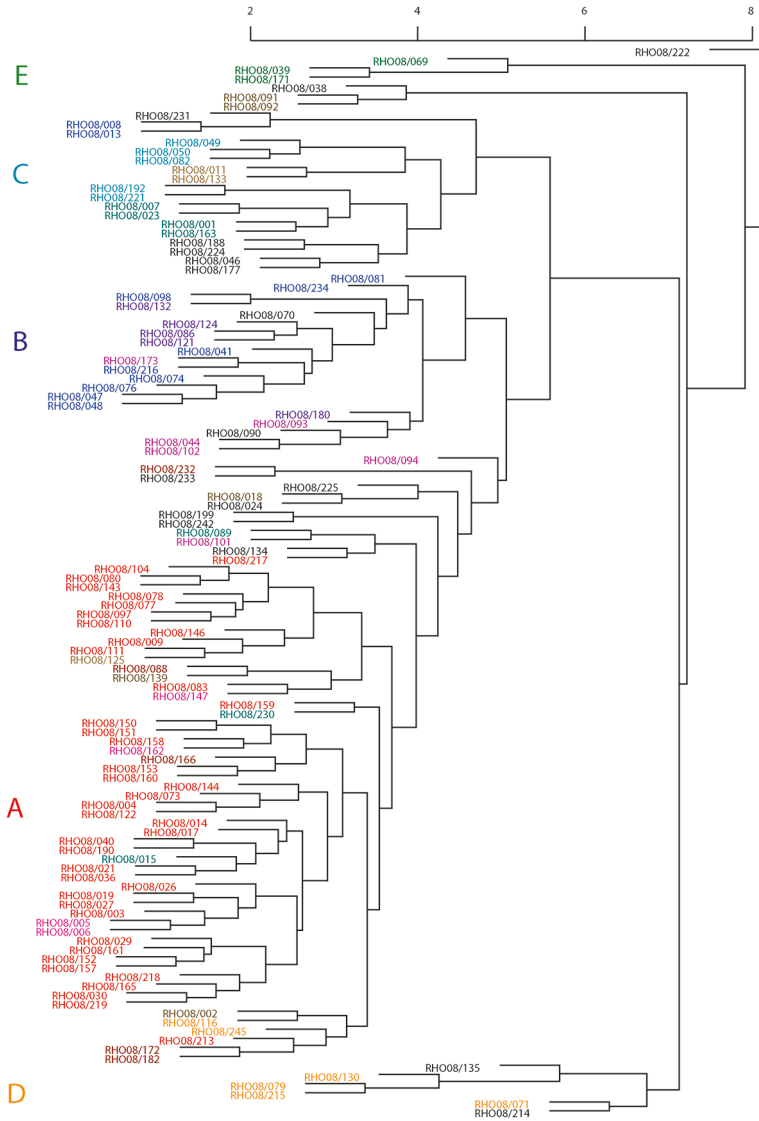
Fig. 7 Hierarchical clustering of 118 NAA measurements of Hellenistic Rhodian amphorae: Concentrations of 17 elements were used, which were log-ratio transformed with the Sm concentration as common divisor. The presented clustering is based on average linkage.
