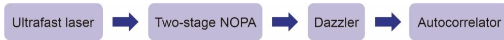
Figure 4.6: Simple scheme of the setup of a two-stage NOPA using a Dazzler for the output compression. The laser pulses are delivered to the two-stage NOPA system and the NOPA output is compressed by Dazzler device and characterized by an autocorrelator.
