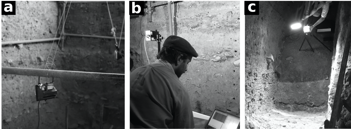
Figure 3.4: Imaging setup during fieldwork. Hyperspectral images, used throughout chapters 4 and 6, were captured using artificial light, which was positioned to create uniform lighting (a). Image acquisition required the hyperspectral camera (Cubert X2 S258) to have a constant wired connection to the imaging software (b). In tight spaces, the usage of a single artificial light source can be necessary (c).
