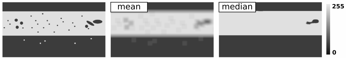
Figure 3.7: Spatial filters applied to an exemplary pixel image (left). The median filter used throughout chapters 4, 5 and 6 eliminates smaller image noise while preserving main features.
