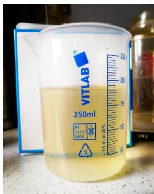
Figure 2.6: Filtered water sample (filtered through 0.22 \mu\text{m} pore size) from a creek runoff draining organic-rich permafrost. The strong yellow colour indicates a high concentration of DOM (Photo: Bennet Juhls).
