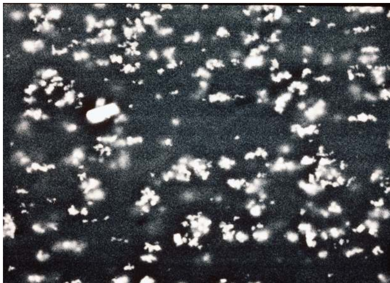
Fig. 3 Micrometer-sized crystals of calcium antimonate in an opaque white glass from a mosaic vessel of the first century. Scanning electron microscope.
