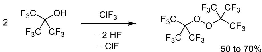
Scheme 1.9. Synthesis of bis(nonafluoro- tert -butyl) peroxide, [(\text{F}_3\text{C})_3\text{CO}]_2 , from the reaction of nonafluoro- tert -butyl alcohol, \text{HOC}(\text{CF}_3)_3 , with chlorine trifluoride, \text{ClF}_3 .
