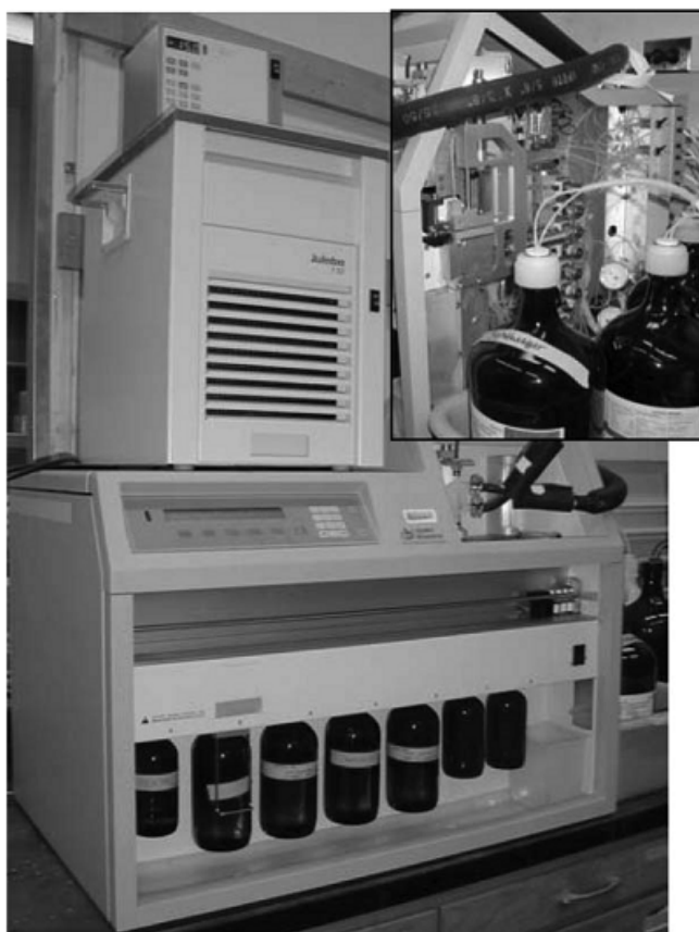
Modified peptide synthesizer used for automated synthesis of oligosaccharides 24
