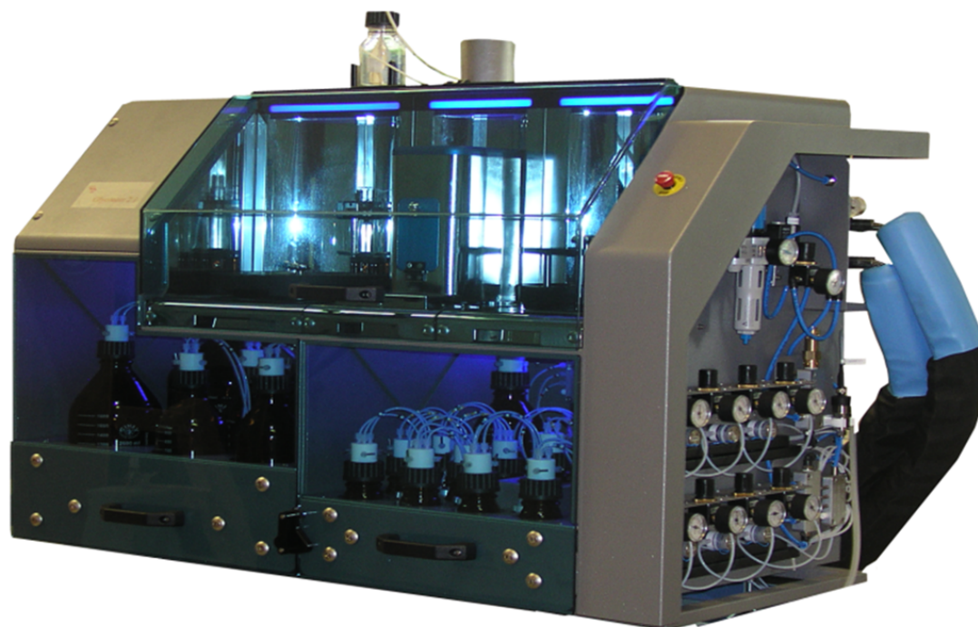
Figure 3: Glyconeer 2.1: The commercially available, automated solid phase oligosaccharide synthesizer
