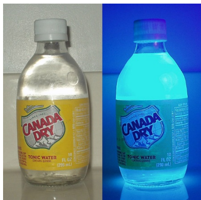
Figure 1: Tonic water, containing fluorescent quinine sulfate, under daylight (left) and under UV light (right). [7]
