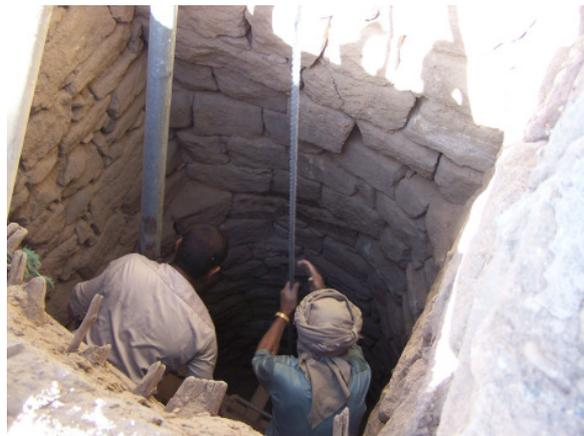
**Figure 4.3:** Sampling by hand from 50 m depth dug well
