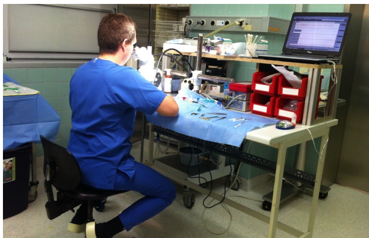
Figure 3a & b - Reinhold, JM. 2013. Murine trauma model working bench (3a, left) and microscopic (surgeon's) view of carotid artery with PE tube in place for invasive blood pressure monitoring (3b, right)
