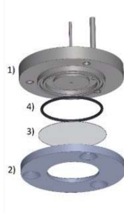
18 19 20 21 22 23 24 25 26 27 28 29 30 31 32 33 Figure S2. Schematic representation of the stagnation point flow model. (1) The top plate with 34 35 inlet and outlet. (2) The stainless steel bottom plate. (3) The transparent (coated) cover slip on 36 37 which the platelet adhesion was visualized. (4) A silicon ring to seal the system. 38 39 40 41 42
