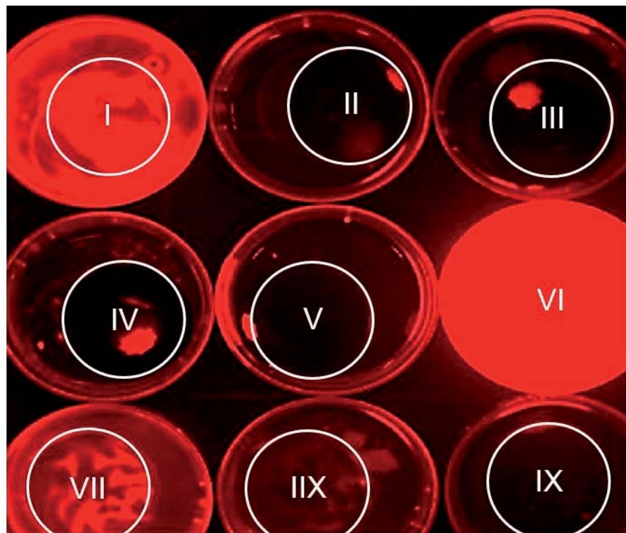
55 56 57 Figure S3. A fluorescence image of bare Ti-substrates and MI-dPG-coated Ti-substrates, 58 59 incubated with TAMRA-amine at various concentrations. The white circles represent the 60 61 62
