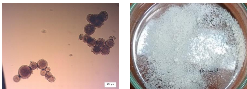
Figure 30 Microscopical (left, scale bar: 100 \mu\text{m} ) and macroscopical (right) appearance of microparticles the primary emulsion of which was prepared by ultrasonication. Microparticles were free-flowing after drying and did not show agglomerates.
