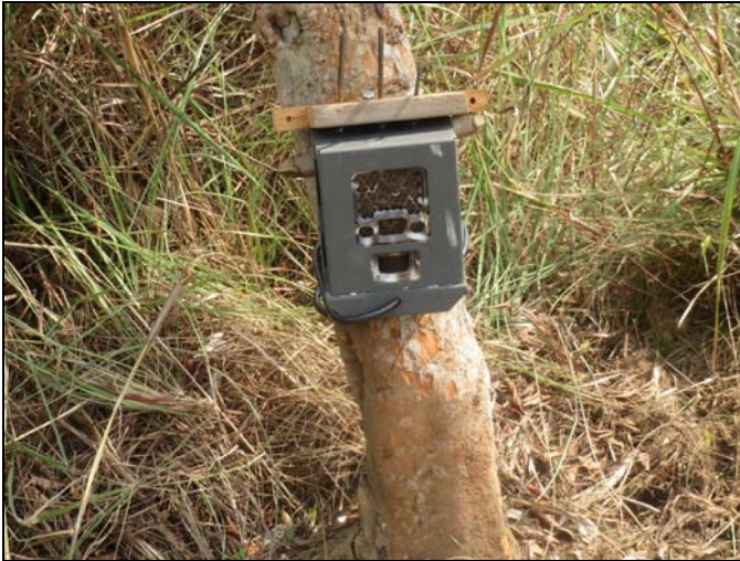
Figure 3. Picture showing camera trap in a security enclosure attached to a tree. For additional security a cable lock was wrapped around the tree and fixed to the security box. Here, additionally, a piece of wood with large nails pointing upwards was attached to the tree above the security enclosure to provide additional security.
