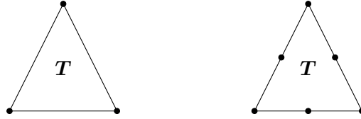
Figure 4.2: A simplicial element \mathbf{T} in 2D with dofs (black circles) for the Lagrange finite elements \mathbb{P}_1 (left) and \mathbb{P}_2 (right).
