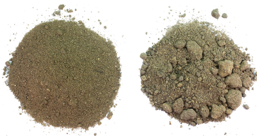
Figure 4.1 Disintegrated (left, MWD=51 \mu m, 29% WSA) and aggregated soil (right, MWD=109 \mu m, 44% WSA) used in the training phase.
