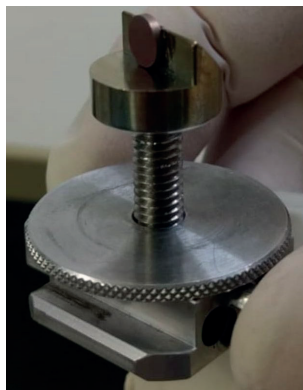
Figure 13. Vertical substrate holder enables the measurement of the coating thickness on the titanium material.
