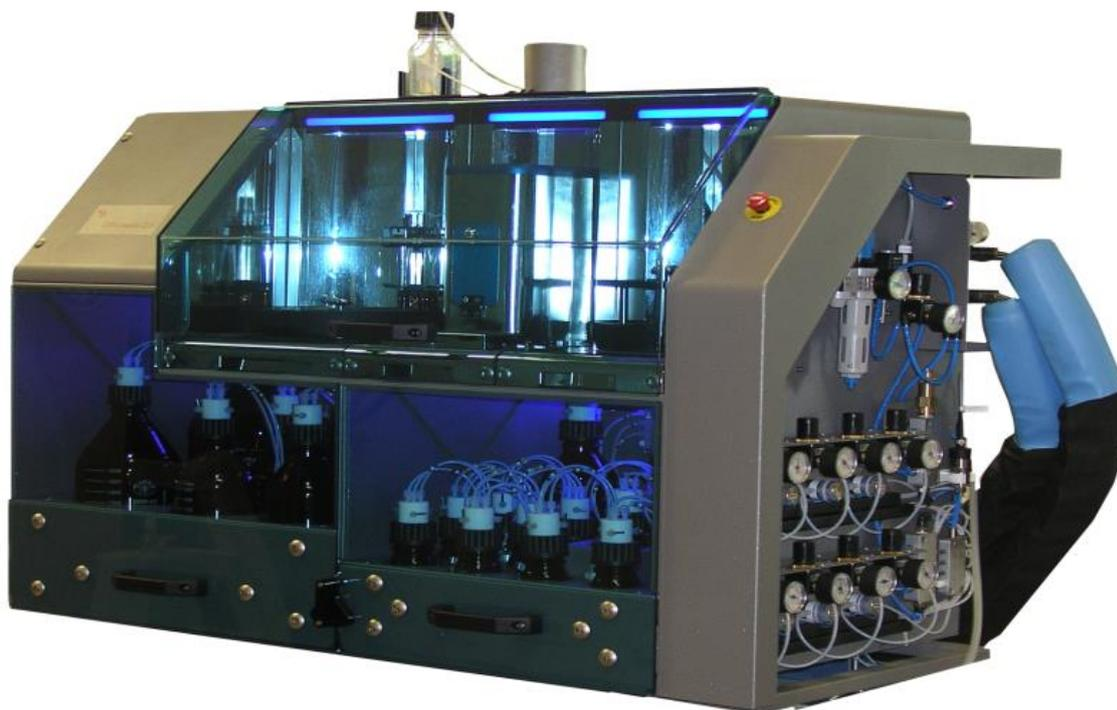
**Figure 1.3** The automated solid phase oligosaccharide synthesizer Glyconeer.
