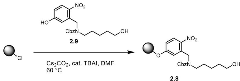
**Scheme 2.9** Functionalization of the Merrifield resin with a photocleavable linker.
