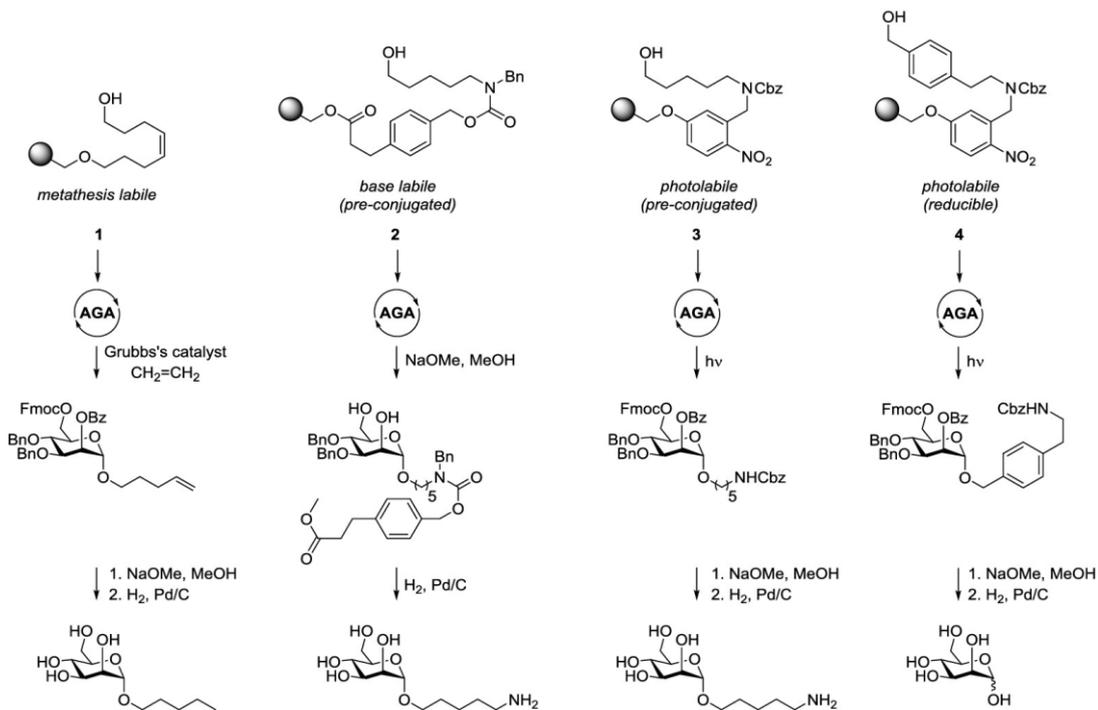
**Scheme 1.3** Linkers for automated glycan assembly. Adapted from ref. 32.<sup>32</sup>
