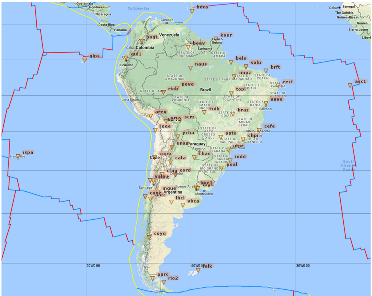
Figure B.4: Location of 56 reference stations used to tie the GPS network solution to the ITRF2014 daily coordinate solution.
